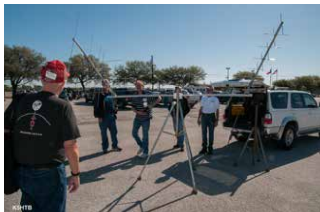
The M-Squared LEO-Pack antennas are carefully balanced for easy aiming, but that is certainly a long boom between the 2M and 70cm antennas. (Travis Burgess, K5HTB photo)
