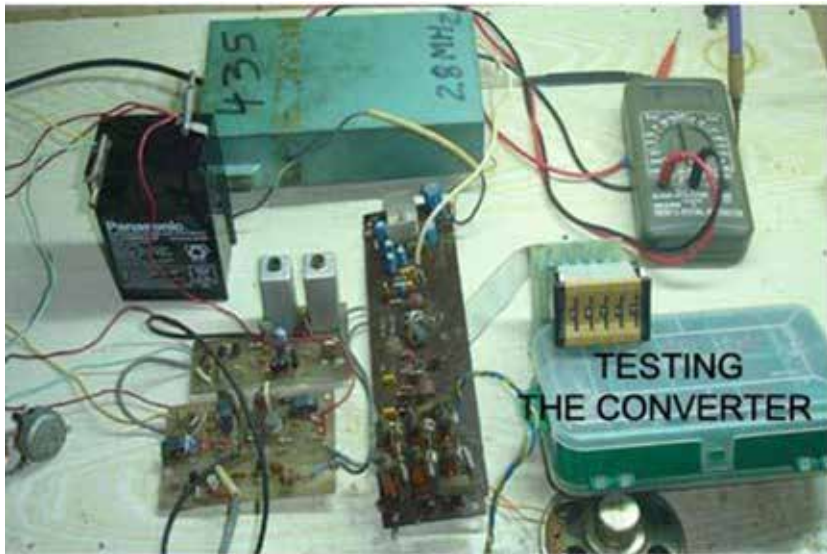
Photo 3: CO6CBF homebrew UHF downconverter
