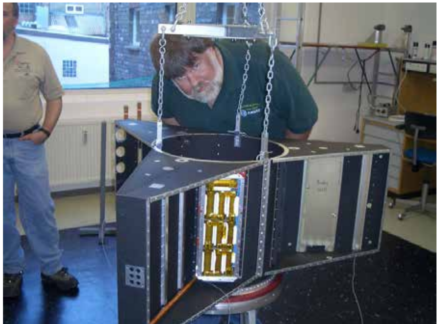
The P3E spaceframe will have room for scientific and amateur radio payload. Bdale Garbee, KB0G, is shown with the spaceframe at AMSAT-DL in 2005.
