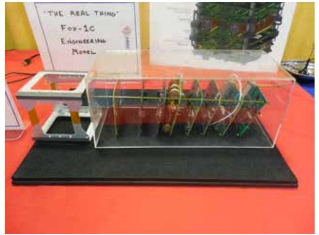
The AMSAT engineering area this year once again included a structural prototype of the FOX-1 satellite, a working model of FOX-1A's transponder and an "expanded" prototype of the FOX-1C spacecraft
