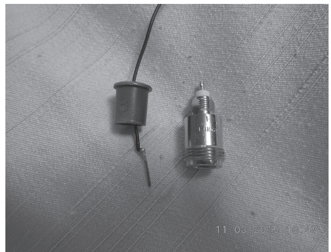
Figure 2 - N connector and plastic cap with wire connection to F connector
