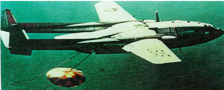
Exposed CORONA film was wound into its upper stage capsule that was later de-orbited and most often snagged in mid-air over the Pacific Ocean by a C-119 cargo plane. [Photo courtesy of USAF.]
