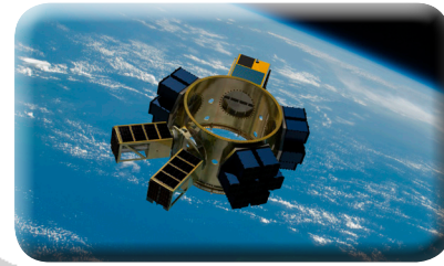
Spaceflight's SHERPA will deploy multiple cubesat payloads on-orbit
