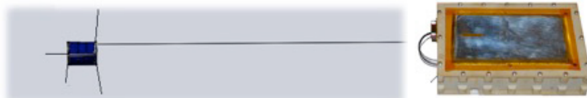
Figure 1 - PSAT-1 with antennas deployed and QIKCOM-2 module with antennas stowed
