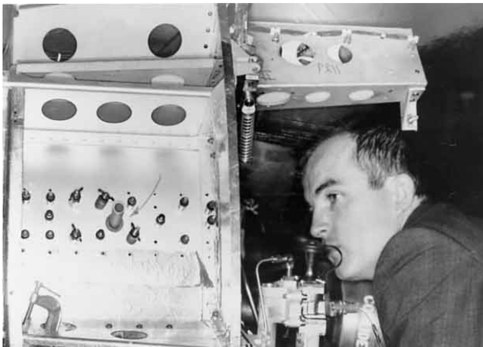
Lance Ginner, K6GSJ, looks over the carrying structure that will loft OSCAR-1 to orbit on the CORONA upper stage. Note the faint arrow pointing to OSCAR-1's $1.15 Sears-Roebuck spring ejection mechanism. [Lance Ginner, K6GSJ, photo.]
