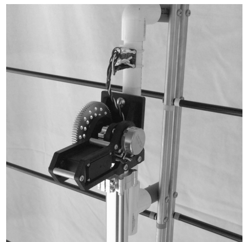
Figure 5 — The elevation gimbal shown with antenna attached.
