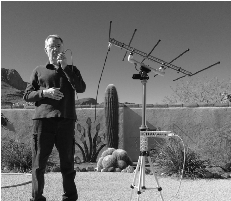
Figure 1 — Tracker gimbal is attached to a tripod and supports an Elk 2m/70cm LPDA antenna.
