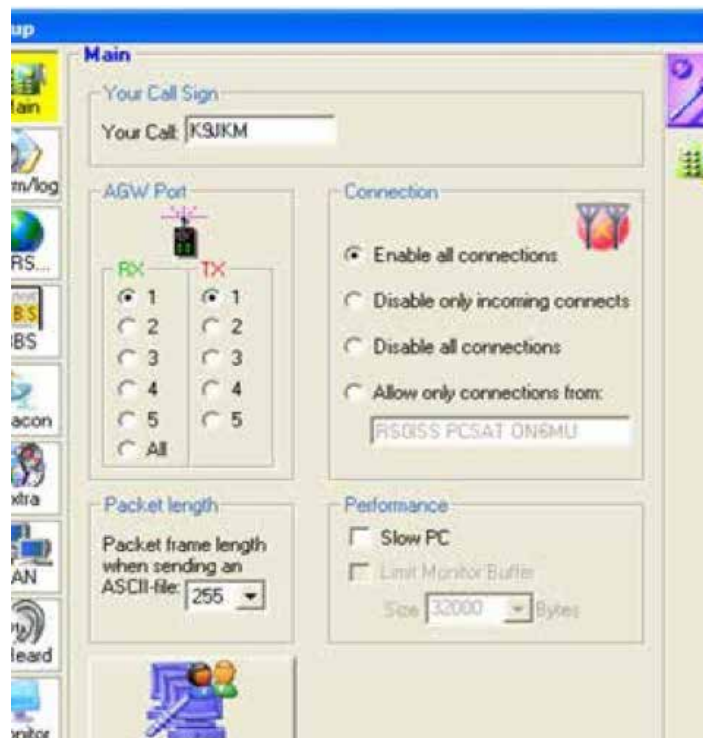
Figure 10 — The UISS program will require settings to be changed to operate with UZ7HO Soundmodem: In UISS top menu, select Setup > UISS > LAN (above screen).
