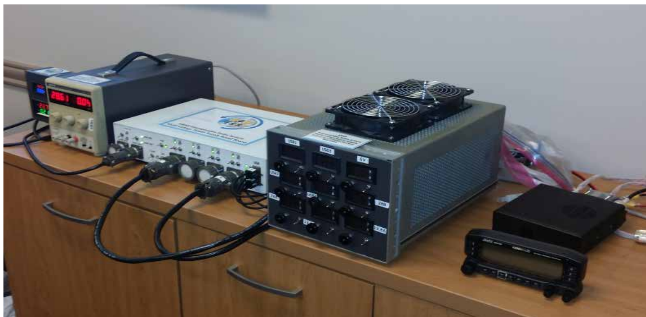
Figure 1 — The Kenwood TM-D710GA radio is shown on the right side of the Interoperable Radio photo. Also, you can see the AMSAT-built power supply (in white) and the load simulators (to the right of the power supply) and power sources to the left of the power supply. [Courtesy of ARISS.]
