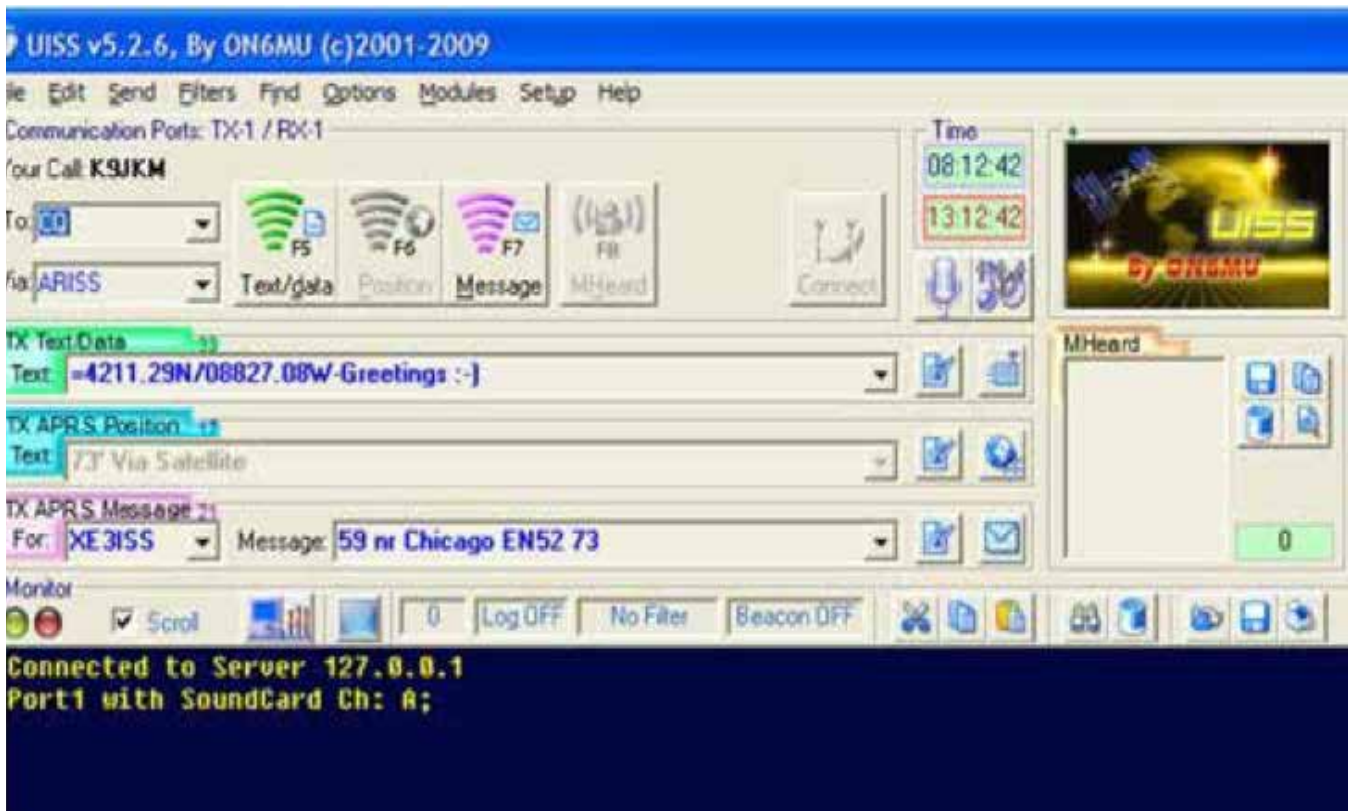
Figure 12 — UISS may prompt you to restart. Go ahead and restart UISS. To return to operation with the AGWPE software, unclick the Enable LAN Mode option and restart UISS. Your setup is now ready for the next ISS pass! To send your APRS position report, click on the UISS Text/Data button. You can enter custom messages for quick packet contacts with other stations into the TX APRS Message box and then click on the Message button.
