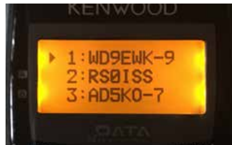
Figure 5 — Station list showing a received position beacon from WD9EWK-9.
