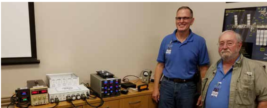
Lou McFadin, W5DID, and Kerry Banke, N6IZW, with Interoperable radio system test set up, including (from right to left) the JVC Kenwood D-710GA, the power supply load simulator, the Bread board multivoltage power supply and the 28 VDC simulated voltage source. [Dave Jordan, photo.]
