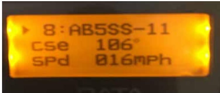
BLT-47 sending telemetry via APRS on 144.39 MHz shortly after launch.
