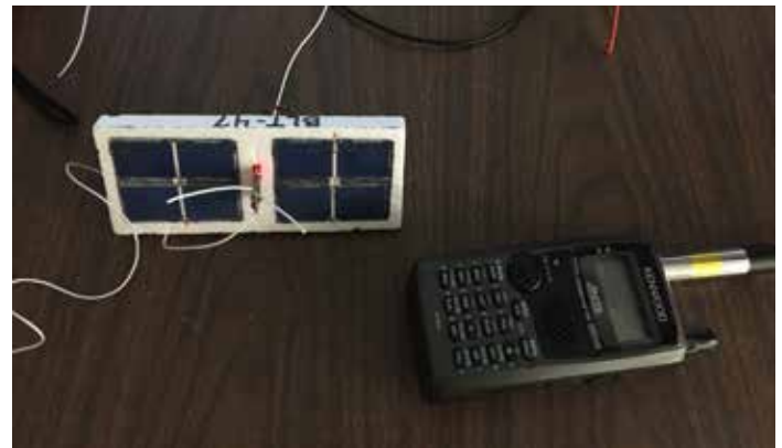
The lightweight APRS system used on BLT-47 (AB5SS-11) adjusts the output frequency appropriately for anywhere on Earth. Solar cells and a rechargeable Li-Ion battery provides 50 mW for an extended period.
