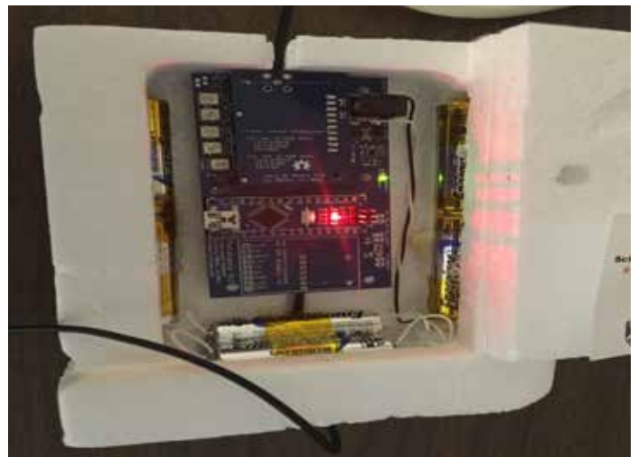
BLT-48’s payload was a miniaturized cross-band FM repeater, 446.000 MHz up and 147.450 MHz down, with 500 mW.
