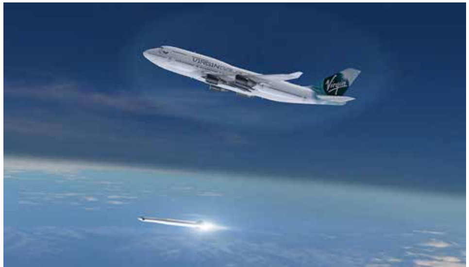
Figure 4 — Virgin Orbit LauncherOne launched from a Boeing 747-400. [Photo courtesy of Virgin Galactic.]
