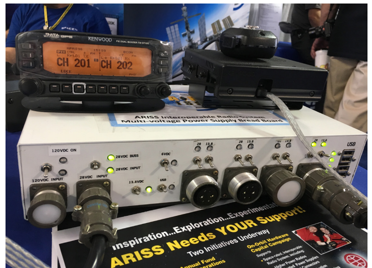
Interoperable power supply with modified Kenwood DM-710G radio. [Joe Kornowski, KB6IGK, photo.]
