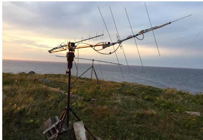
In recent years, M2 Antenna Systems has marketed their “LEO Pack” consisting of their Model 436CP16, circularly polarized Yagi for 70cm and their Model 2MCP8A, circularly polarized Yagi for 2m. The array is shown here being used during a recent DXpedition to St. Paul Island, Canada. [CY9C, photo.]
