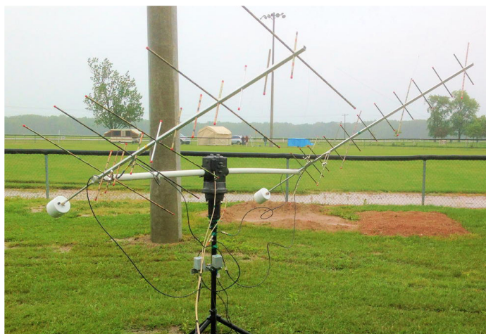
ARRL’s Field Day is a great opportunity to try out different portable satellite antenna designs. Here, a pair of Arrow-style antennas are used with 75 Ohm phasing lines to achieve a “circular-like” radiation pattern. The rotator is a Yaesu G-5400 Az/El combo and the tripod is a DJ speaker stand, both obtained from E-Bay.
