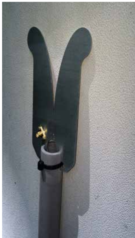
Figure 6 — RFSpace UWB-4 Vivaldi antenna used alone; PVC + a wire tie makes an excellent mount.
