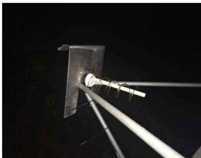
Figure 4 — L-band Helical Dish Feed made from #10 copper wire with PVC support (easily removable as dish is used with many different feeds).
