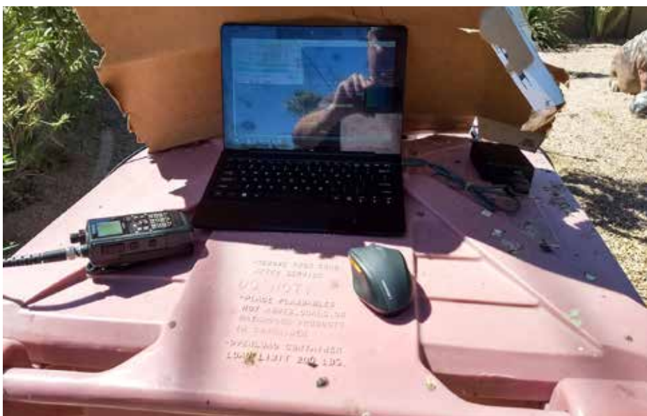
"Frankenstation" using TH-D74 with SDRplay RSP1.
