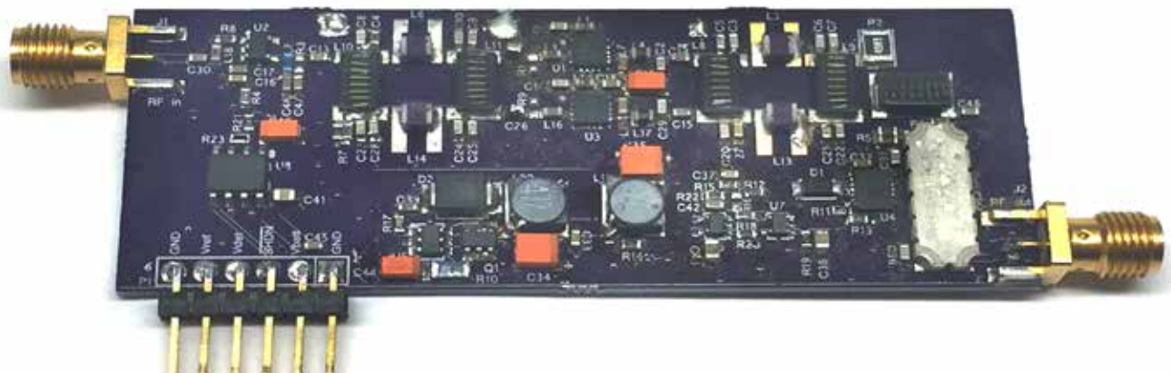
Fig. 8 — Photograph of the prototype using two RF power amplifiers in quadrature, a driver stage, a low pass filter and a directional coupler. The power control circuitry is located at the bottom of the board.
