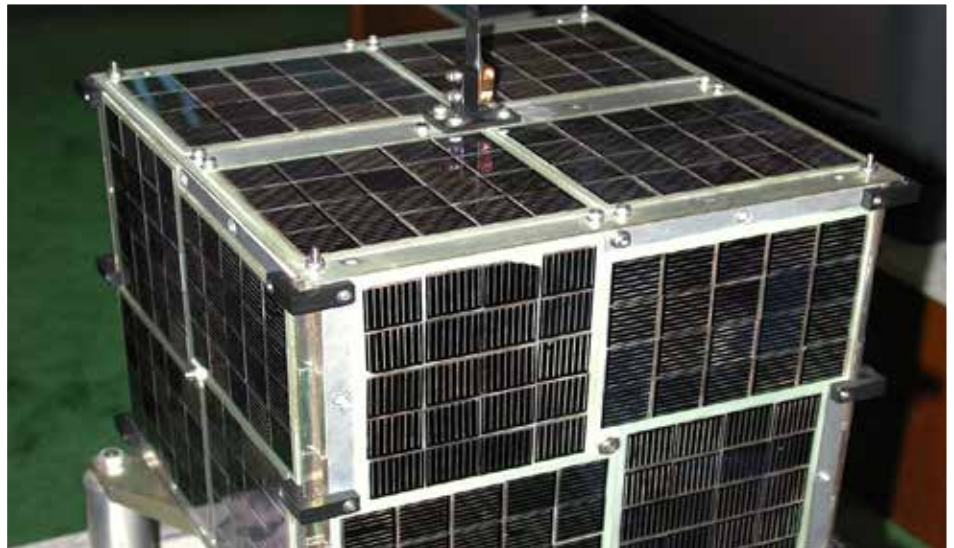
A close-up photo of a completed MicroSat showing its solar panels.
