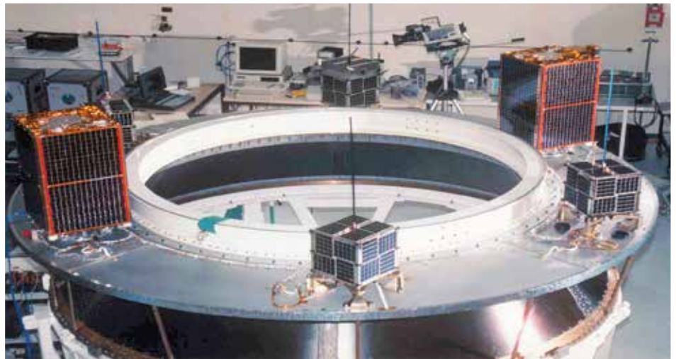
Dove satellite (far right) sits on its "Ariane Structure for Auxilliary Payloads" (ASAP) launch structure with three other MicroSats and two UoSats.
