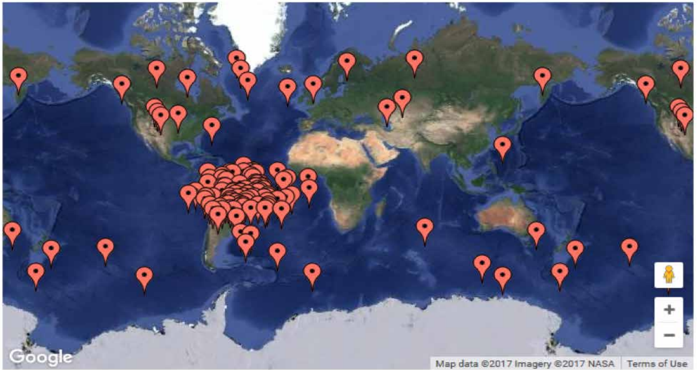
Figure 1 – The map of satellite subpoints for AO-85 CPU reset numbers 0 through 713. An interactive version of this map appears online at qsl.net/ka2upw/ao85_reset_map.html , but eventually, I would like to get the map and scripts onto the AMSAT website.
