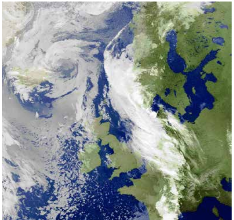
Figure 3 – MCIR (“map coloured infrared”) enhancement of APT signal.
