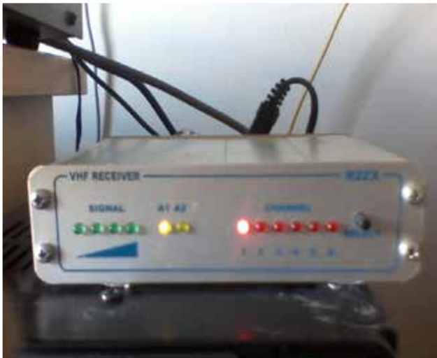
Figure 1 – The R2ZX receiver for APT on 137 MHz.
