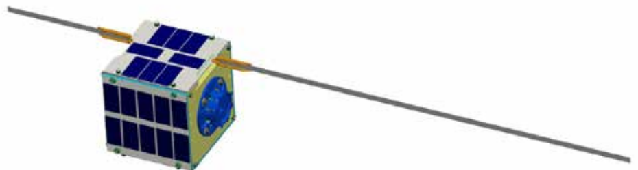
An artist's concept of the CAS-3F (XW-2F) satellite. For size comparison, the longer whip is the 1/4 wave 2 m downlink antenna. [Courtesy: CAMSAT.]
