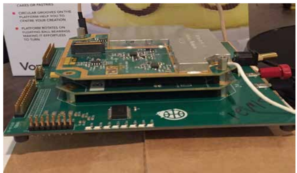
Figure 3 – Turntable and IHU/Rx/Tx Setup (Tx is below the breakout board).
