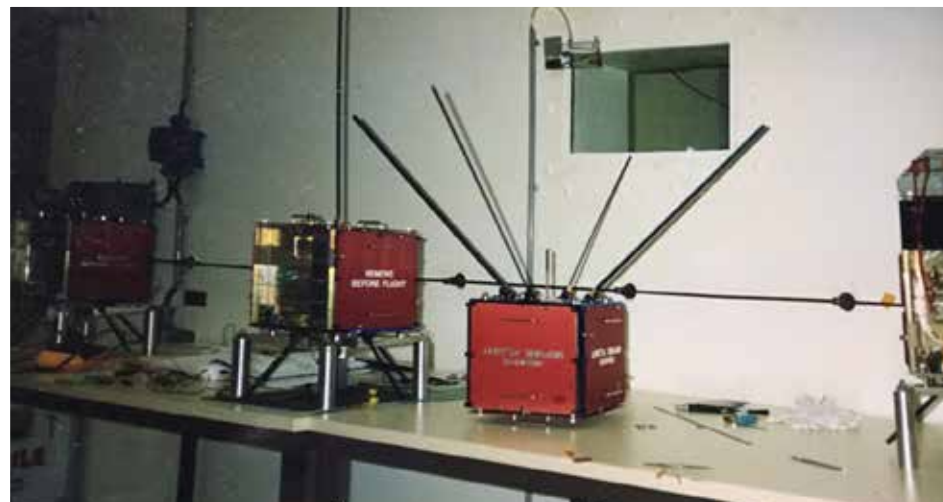
Junior's completed "Dove" satellite (which later became DO-17 on orbit) sits inverted prior to final integration with its launching structure.
