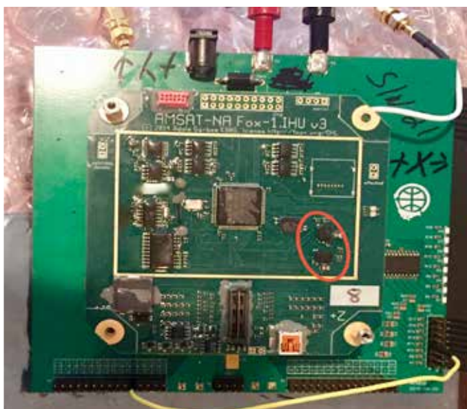
Figure 1 – A Fox-1 IHU On A Breakout Board With Gyros Circled.
