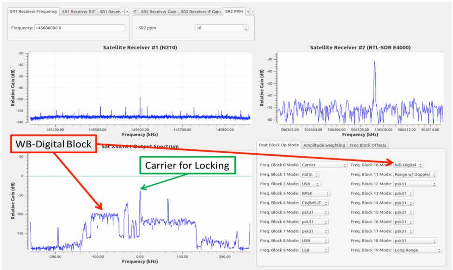
Figure 4-2 Satellite receivers enabled, one tuned to 2 meters, the second tuned to an ATSC HD pilot tone.
