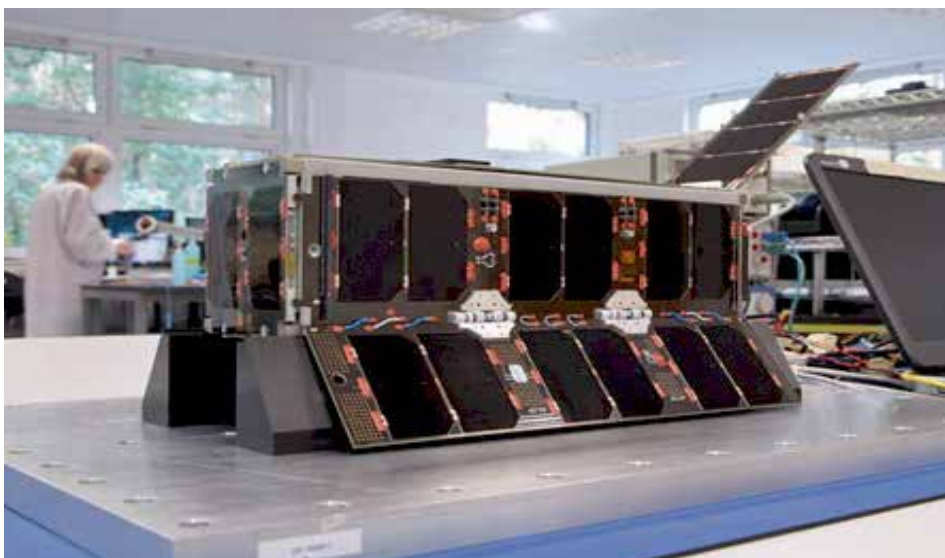
Figure 2 - UKube. 3U CubeSat with deployable solar panels at ClydeSpace 2013.
