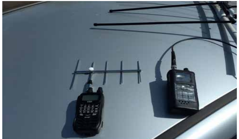
Closeup of Alinco DJ-G7T with Comet CY-1205 1.2 GHz Yagi, Kenwood TH-D74 with Elk log periodic. This pass favored the west coast.
