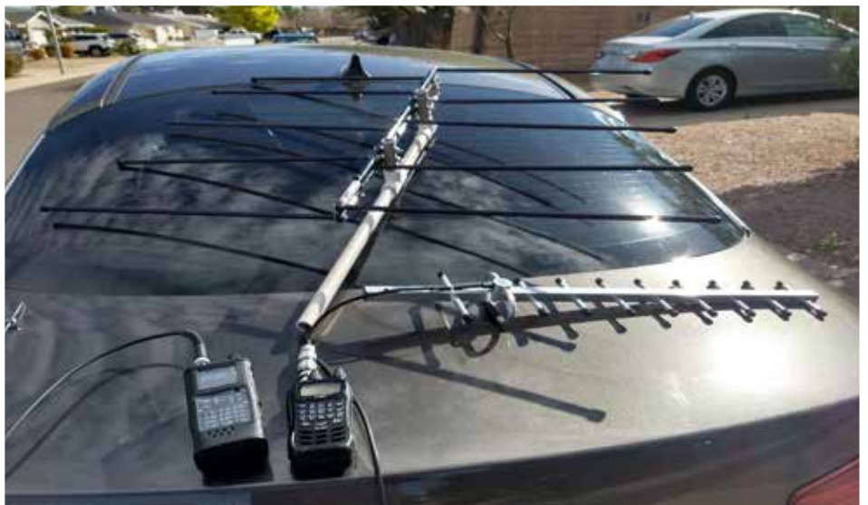
Kenwood TH-D74 connected to Elk log periodic, Alinco DJ-G7T connected to 10-element 1.2 GHz
