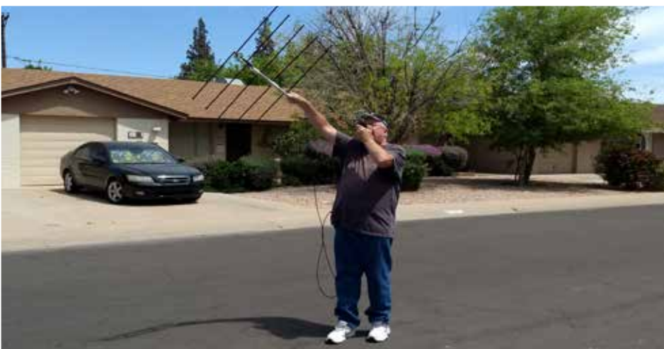
WD9EWK standing in front of his house, working AO-92 L/V. The DJ-G7T is in his left hand, with the Comet CY-1205 Yagi. The Elk log periodic is in his right hand, connected to a TH-D74 on his belt. This pass favored the west coast.
