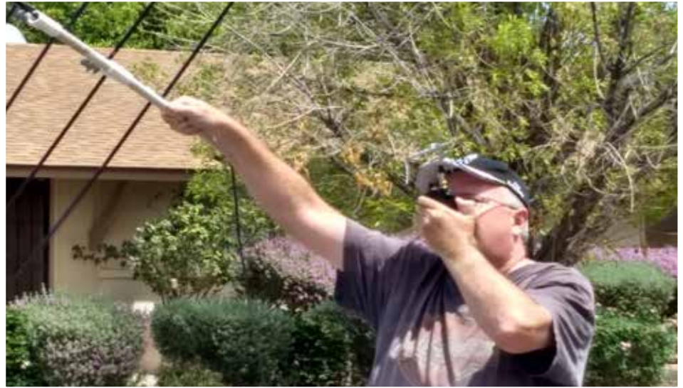
WD9EWK holding Alinco DJ-G7T HT with Comet CY-1205 5-element Yagi in left hand and Elk log periodic in right hand (onnected to TH-D74 clipped on belt).
