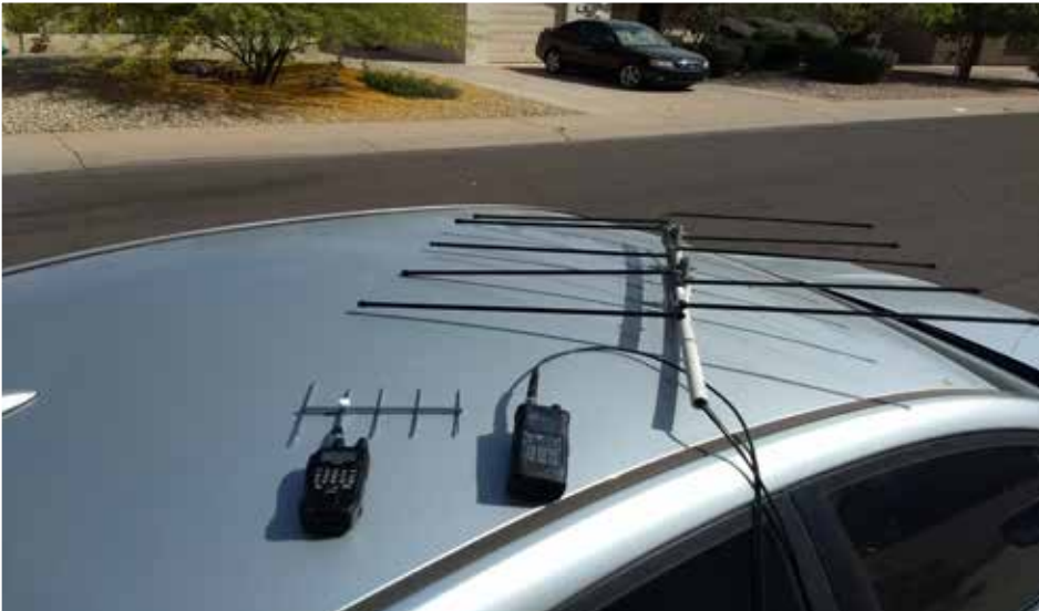
Alinco DJ-G7T with Comet CY-1205 1.2 GHz Yagi, Kenwood TH-D74 with Elk log periodic
