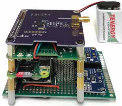
Figure 5 — Proof of concept prototype stack.
