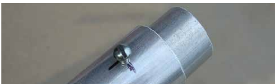
Figure 7 — If it is necessary to tune the antenna to a lower frequency, adjustable sections can be added to each dipole element.
