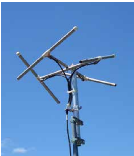
Figure 1 — 2-meter Lindenblad used for our ARISS backup station.
