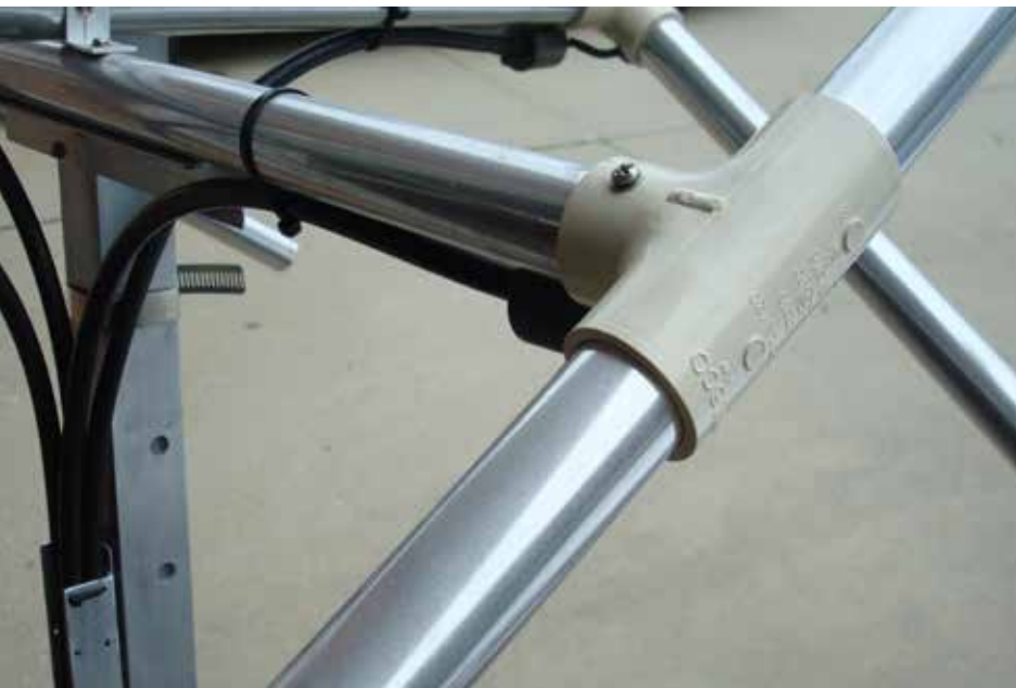
Figure 3 — Machine screw on top of insulator holds dipole at 30 degrees from horizontal.
