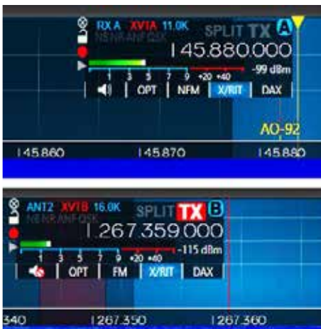
Figure 3 — FlexRadio SmartSDR Slice Flags showing actual frequencies.
