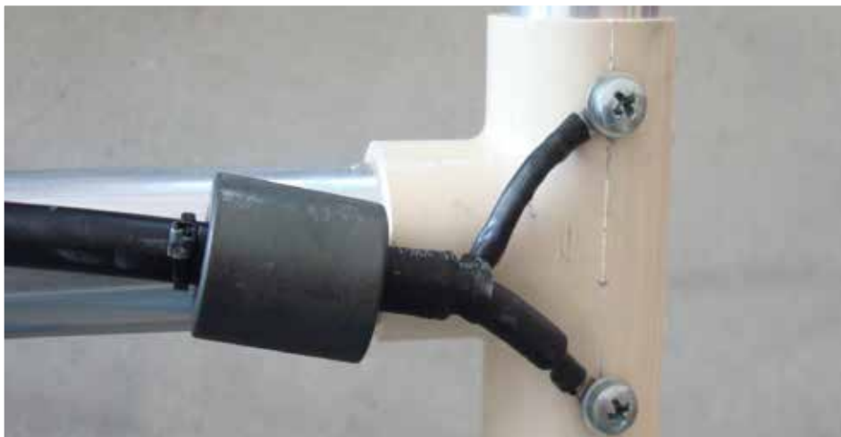
Figure 6 — CPVC tee fittings serve as center insulators for dipole elements, here viewed from the bottom of the antenna.
