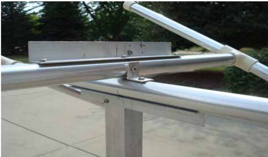
Figure 2 — Crossarms are connected to the mast using short pieces of \frac{3}{4} ' aluminum angle stock and machine screws.
