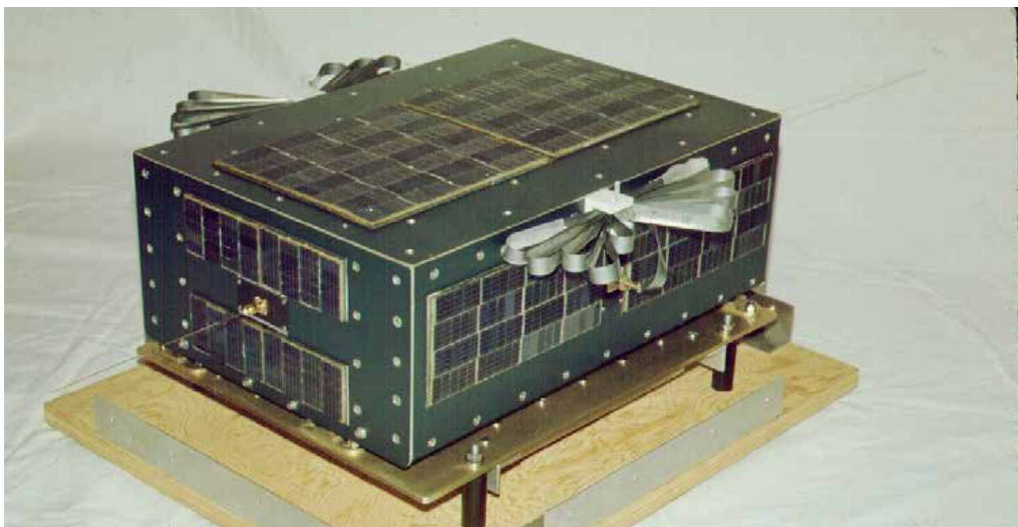
OSCAR 6 complete. Note the tape measure antennas on the sides for the 29 MHz half-wave dipole.
