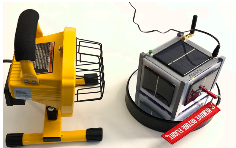
Figure 3 — The CubeSat Simulator on a rotating turntable under halogen work lamp illumination.
