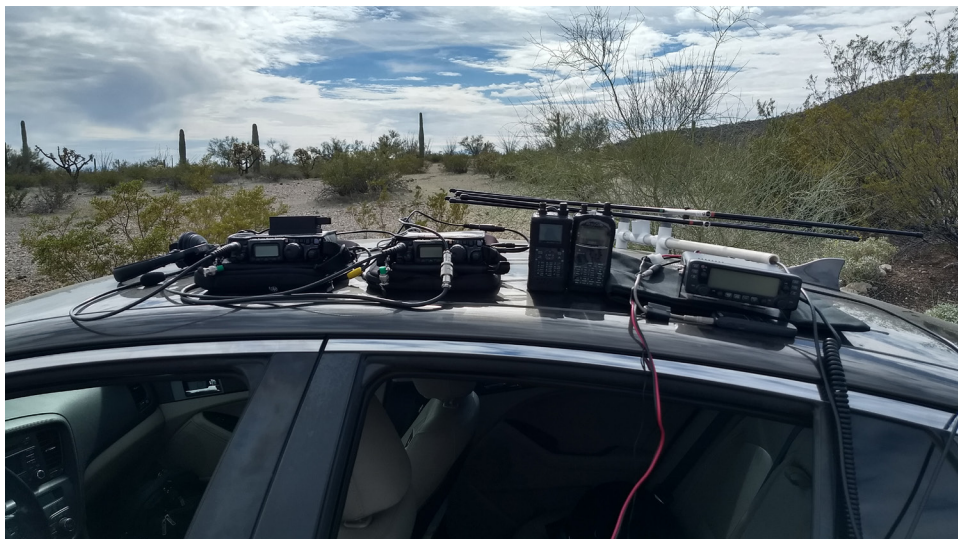
The author's portable station: 2 Yaesu FT-817NDs, Kenwood TH-D74 and TH-D72, ICOM- 2730, Elk log periodic antenna.
