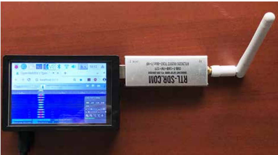
Figure 12 — Raspberry Pi Ground Station running OpenWebRX with Touch LCD Display.
