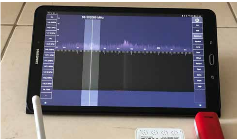
Figure 14 — No-Install RTL-SDR with Android, running SDR touch application.
