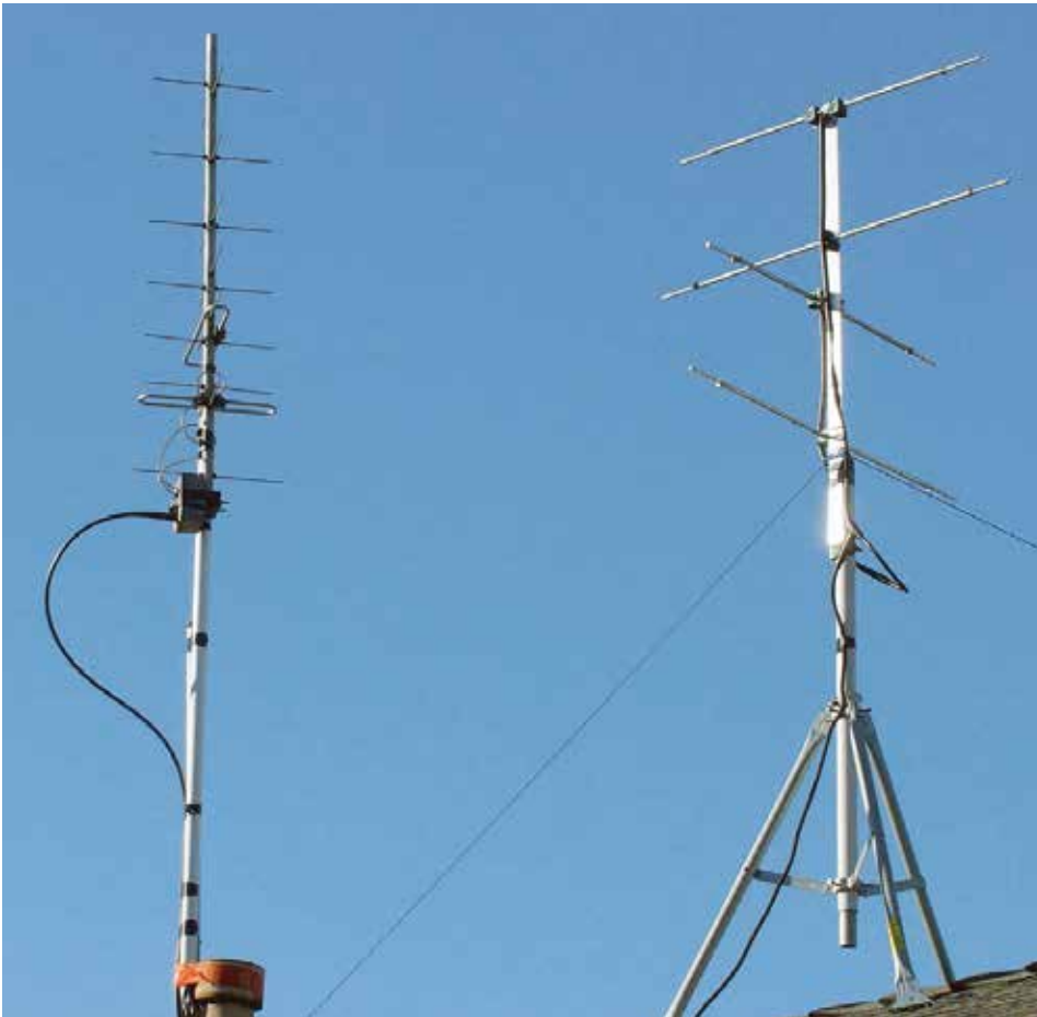
Figure 3 — Installing a pair of antennas pointed straight up yields big signals when satellites pass directly overhead. [Courtesy: ARRL]
