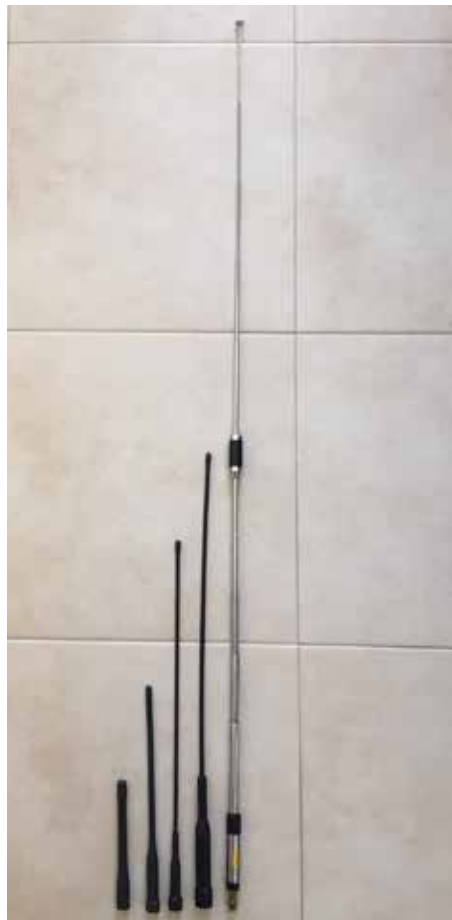
Figure 1 — Wouxun stock duckies, Nagoya NA771, Nagoya R3 and Nagoya RH-770. [Pedro Sousa, CU2ZG, photo.]
