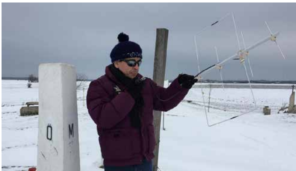
Figure 2 — Open Sleeve Short Moxon. [Pedro Sousa, CU2ZG, photo.]
