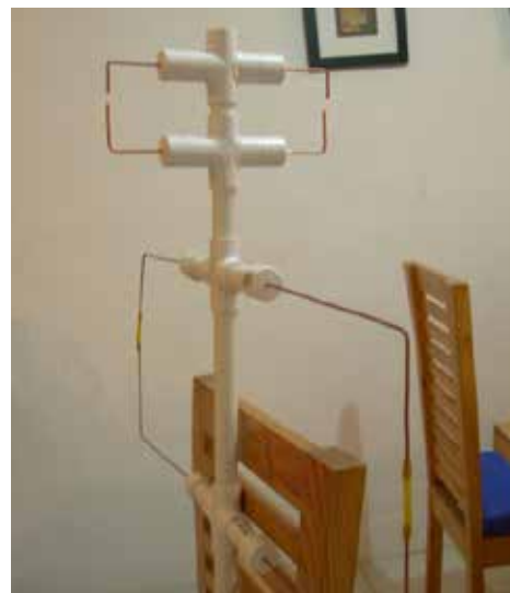
Figure 5 — VHF and UHF antennas made by XE2O.
