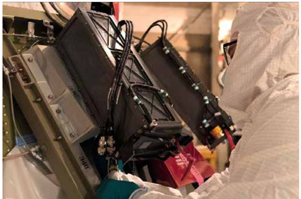
A worker bolts one of the three "PeaPod" carrying structures, one of which successfully carried AMSAT's Fox-1B satellite (now AO-91) to orbit to the upper stage of its Delta II rocket. (Courtesy: NASA)
