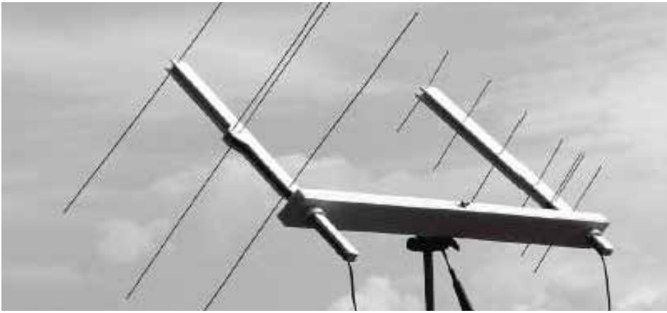
Satellite antennas don't need to be fancy to be effective. Here, a pair of vertically polarized, homebrew Yagi antennas made from bits of wire and wood are mounted on a wooden cross boom. (Courtesy: AMSAT)
