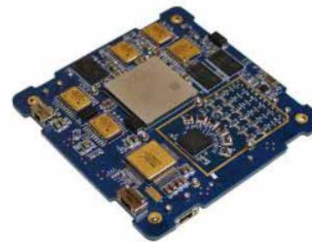
Figure 4 — AstroSDR from Rincon Research Corporation. The board contains a software-defined radio (SDR), FPGA signal processor, ARM processor, and data storage.
