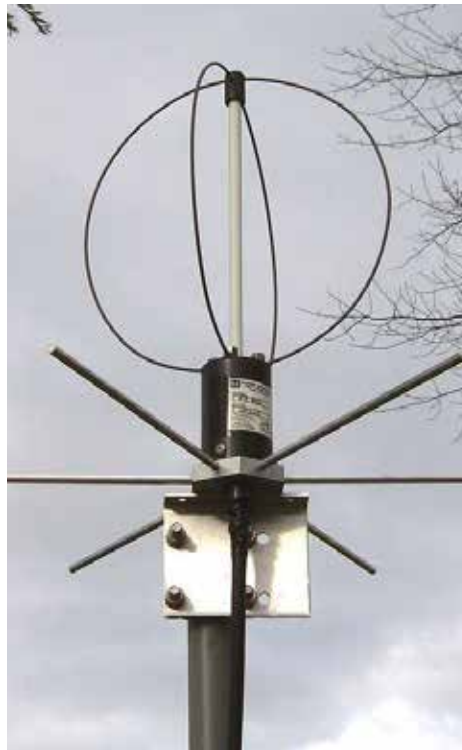
This photo shows a view of the author's 70 cm, M2 "Eggbeater" antenna. Note the ground radials mounted underneath the phasing coil. (Courtesy: KB1SF)
