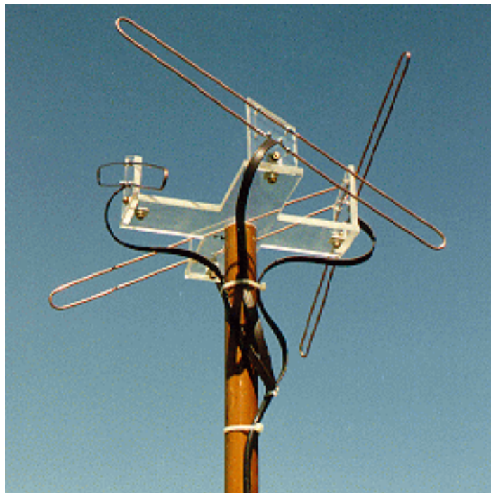
The Lindenblad antenna is yet another, relatively easy to build omnidirectional antenna suitable for satellite work. (Courtesy: AMSAT)
