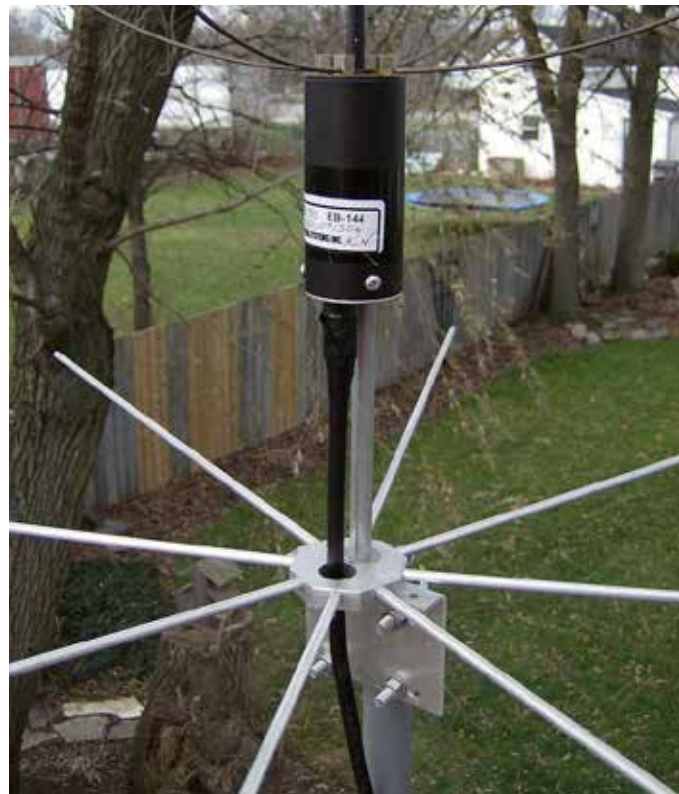
Here's a partial view of the phasing coil and ground plane of the author's 2m, M2 "Eggbeater" antenna. Note that the ground plane radials are offset by about 1/2 wavelength (10.5 inches) from the top of the phasing coil and driven elements. (Courtesy: KB1SF)
