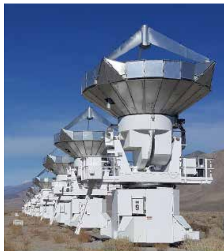
Figure 1—Arizona Array Antennas. Each antenna is a fully steerable, 6.1 meter parabolic reflector that can operate up to ~300 GHz.
