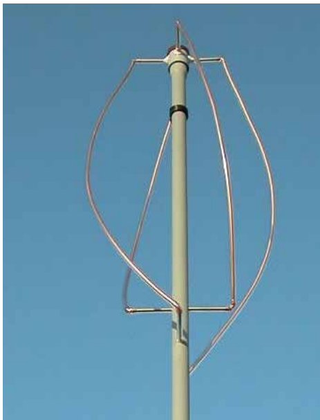
The Quadrafililar Helix antenna is a relatively easy to build omnidirectional antenna that can be optimized for both amateur radio and weather satellite work. (Courtesy: Bob Cash, N8IMO)
