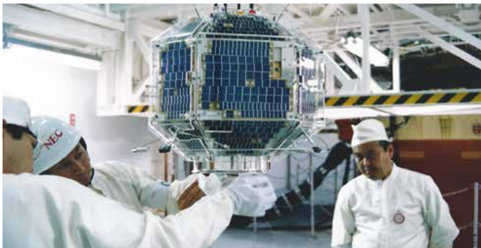
Technicians make a final adjustment to JAS-2's (FO-29's) upper stage attachment mechanism just prior to the final integration and eventual launch of the satellite. (Courtesy:JARL)
