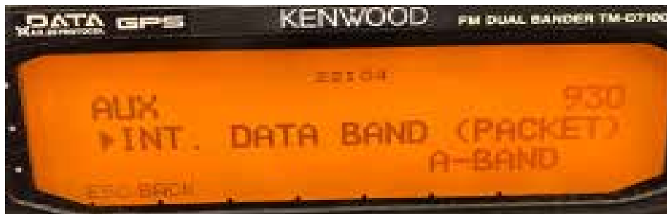
Figure 5 — Display with Squelch Set Up Properly and Downlink Signal Present.
