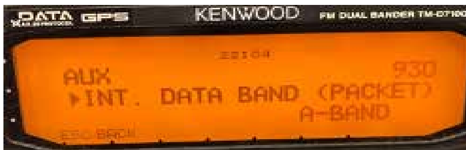
Figure 4 — Internal TNC Set for Full Duplex.
