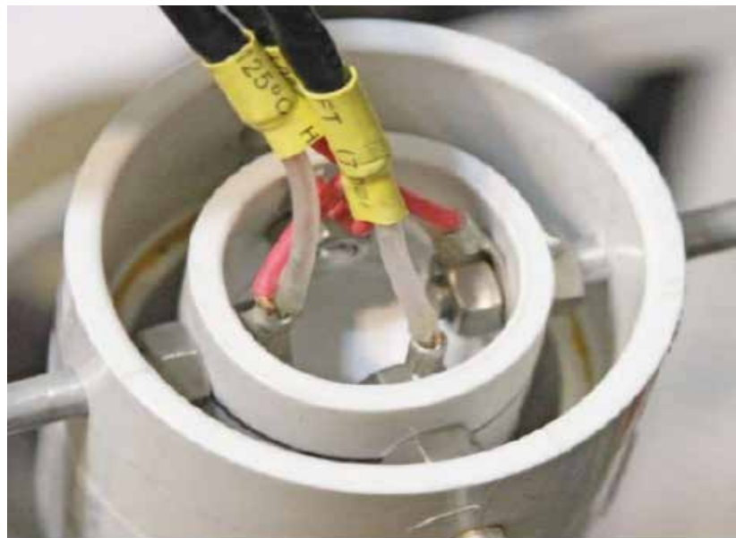
Figure 3: QFH feed point assembly. [David P. Finell; Build a 2-Meter Quadrifilar Helix Antenna , 9 July 2019].
