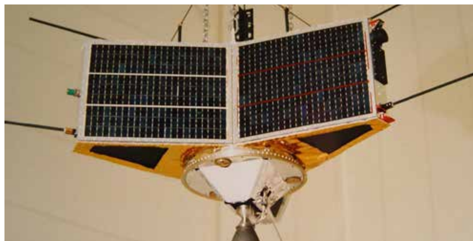
AMSAT-Germany's Phase 3-C satellite (which later became AMSAT OSCAR 13 (AO-13) on-orbit) was a very popular linear transponder satellite that provided amateurs with near worldwide coverage before its (unplanned!) de-orbit in late 1996. (Courtesy: AMSAT-DL)
