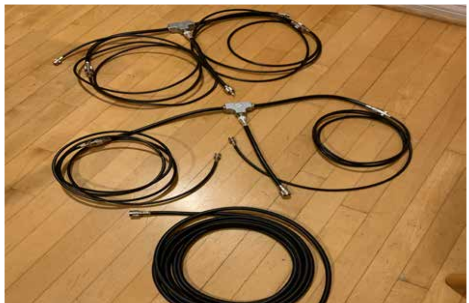
Simple setup for phasing cables.
