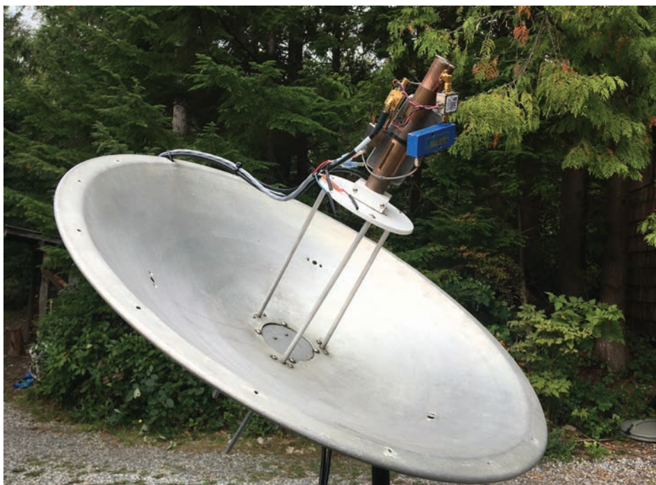
Figure 1 – A view of the 66cm Deep Space Network (DSN) antenna located in VE7TIL's backyard. (All images are credit Scott Tilley VE7TIL unless otherwise noted.)
