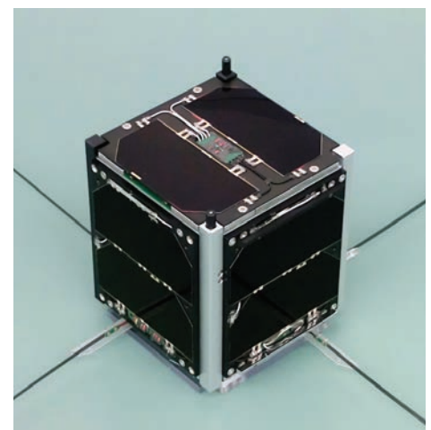
Figure 5 — The flight model of FUNcube-1 (AO-73) is shown here with its VHF and UHF antennas deployed. (Courtesy: AMSAT-UK)
