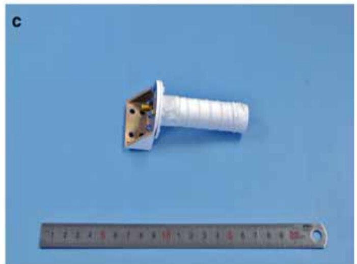
a Block diagram of VHF/UHF radio. b Flight hardware of the VHF/UHF transceivers and miniature CMOS camera. c Flight hardware of a VHF/UHF dual-band antenna.
