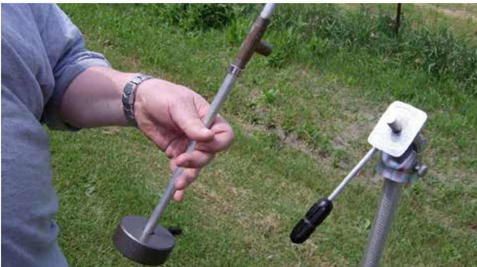
Here's the basic Gizmo with the counterweight, main shaft and plumbers Tee and bushings installed. Note the drill stop between the Tee and the weight. This addition is not necessary but Art finds it handy so that the shaft doesn't slide in the Tee when attached to the antenna. Also note the short stub attached to the tripod. (Courtesy: Author)
