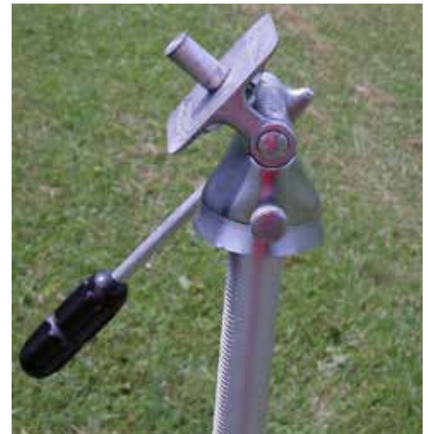
The short stub screwed into the tripod head set to about 45 degrees. The angle of maximum elevation of the upcoming satellite pass is set with the tripod's elevation control. (Courtesy: Author)
