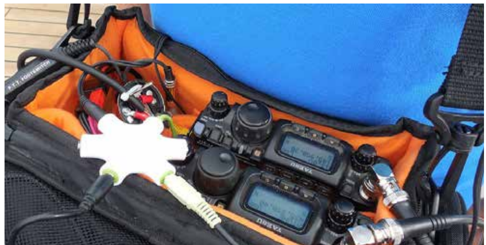
Frank mounts his two Yaesu FT-817s along with a Gel-Cell battery inside a nylon camera bag strapped around his neck. (Courtesy: Author)
