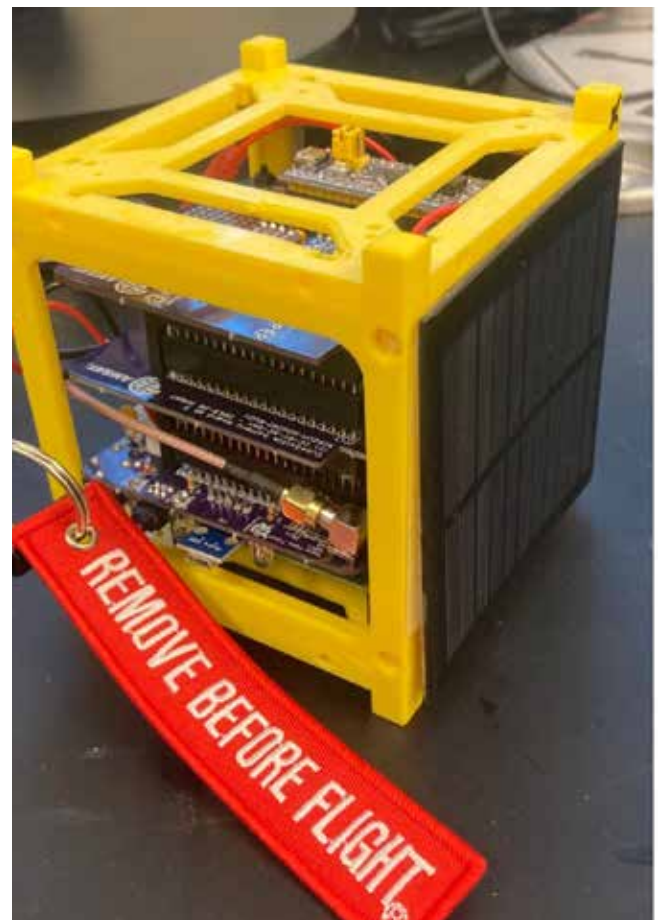
Figure 4 — Completed build with solar panels and frame attached.
