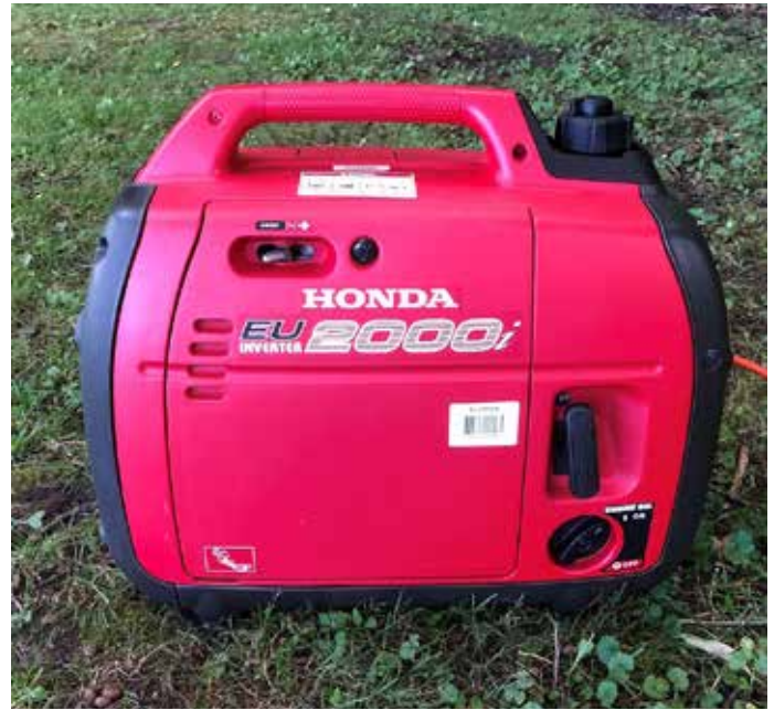
If you plan to operate “off the grid” for an extended period of time (such as at a camp site without access to AC power) a small, portable, gasoline powered, AC generator can provide power for your larger satellite radios and/or recharge your portable batteries, often at the same time! (Courtesy: Author)
