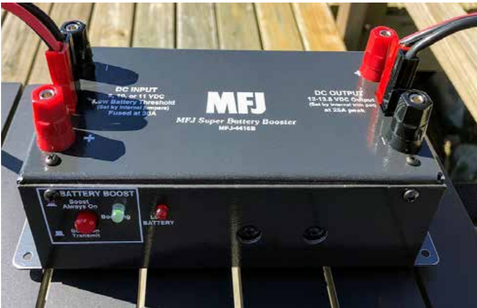
A “battery booster” (similar to this MFJ Model 1441) helps keep your radio’s input voltage steady by eliminating low or marginal voltages from your battery while it’s under transmitting load. (Courtesy: Author)
