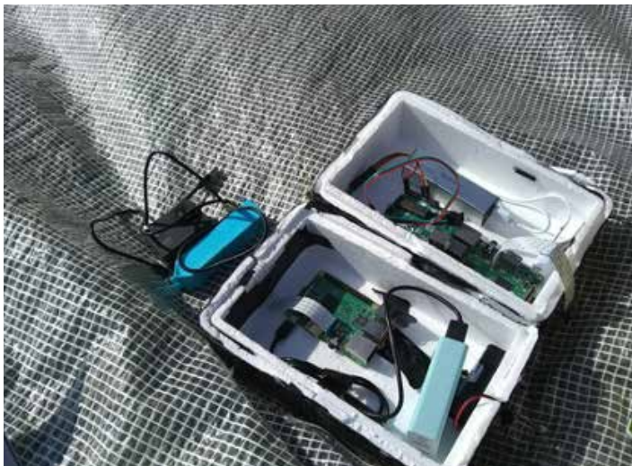
Figure 16 — A payload using Raspberry Pi boards, micro:bit sensors, cameras and powered by mobile charging batteries and AAA lithium batteries.
