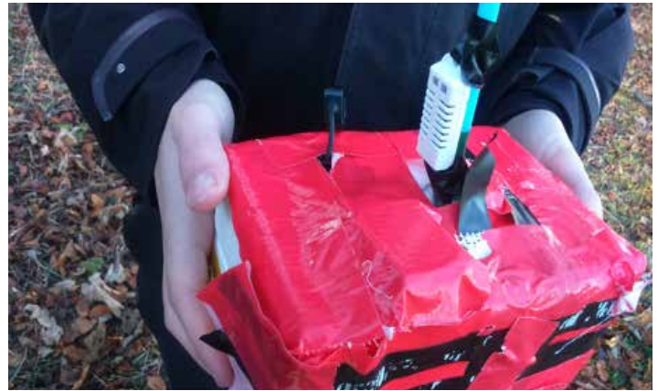
Figure 11 — Students from St. John Henry Newman School in Stevenage mounted sensors on the outside of the box to gather data on UV, temperature, pressure, and a camera took photos with data saved to the Raspberry Pi.
