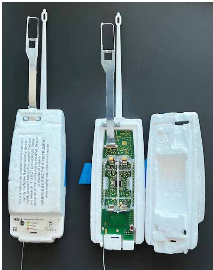
Figure 1 — Recovered NOAA National Weather Service RS41 Radiosonde, reflashed for amateur radio HAB use.
