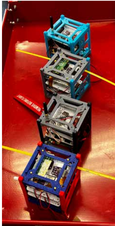
CubeSatSims built by freshman electrical and computer engineering students.
