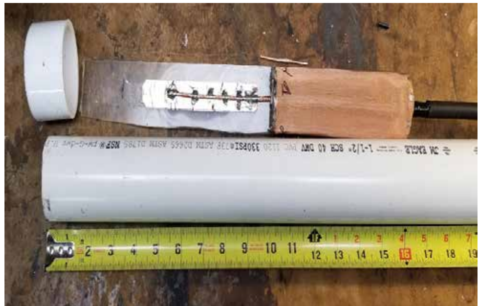
Figure 17 — The sleeve dipole antenna before insertion in a length of PVC pipe. The lower half of the dipole (right side of the photo) is a large cylinder made from a copper screen. The coax braid and screen are attached at the center of the dipole. The center conductor of the coax connects to copper foil, supported by Lexan (top left side of the photo).
