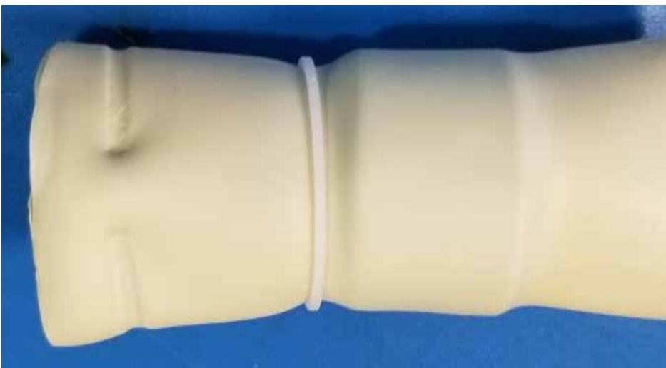
Figure 23 — Valve inserted into balloon neck. Note the white retainer ring is slightly smaller than the valve outside diameter.
