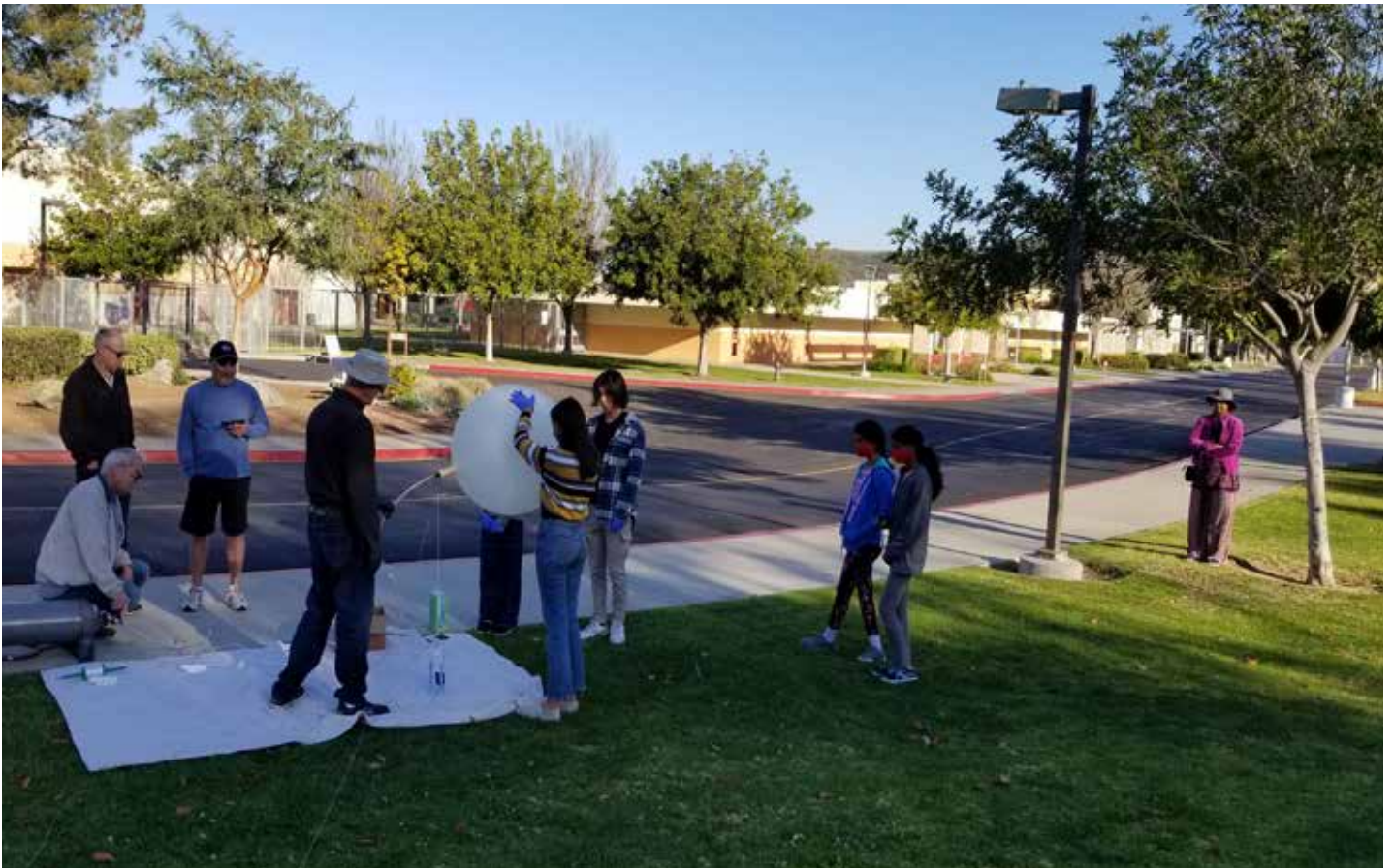
Figure 25 — MCHSARC students filling a 200 g balloon. Note dual sonde payloads on the left side of the tarp. One transmits 4FSK for tracking, and one runs experimental software with a custom camera.
