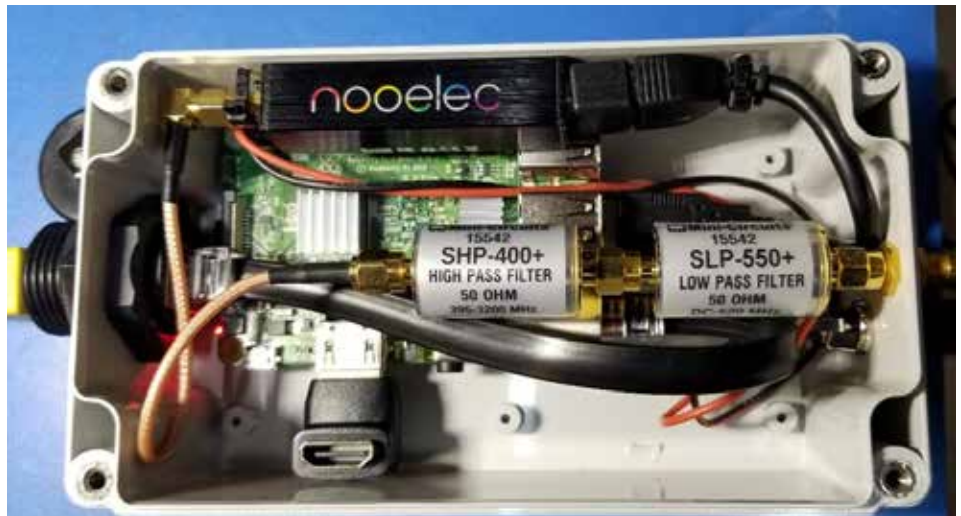
Figure 7. A dual-mode ground station is built into a protective enclosure.
