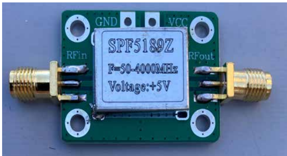
Figure 14 — SPF5189Z preamp "fixed" by replacing the fake SPF5189Z part.
