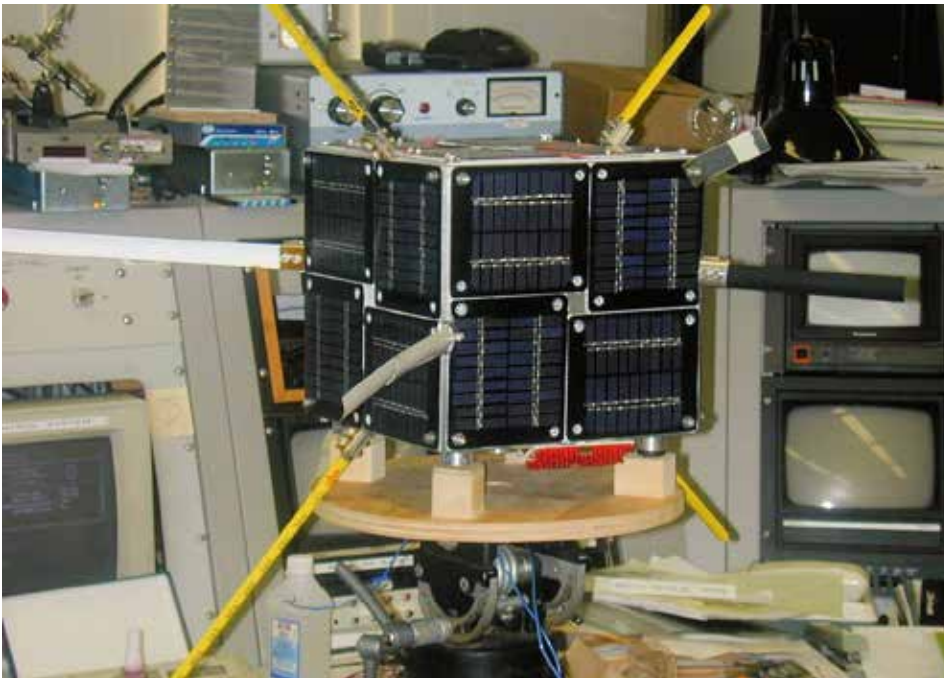
The flight model PCSat is shown here in the U.S. Naval Academy Lab. Note the two black and white painted tape antennas. These are used much like the little sun-powered radiometers we often had as children to give the satellite an approximate 1 RPM spin on orbit. (Courtesy: USNA)
