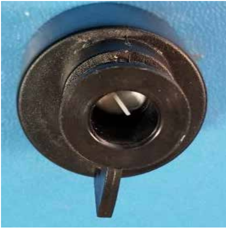
Figure 19 — Valve external to the balloon.
