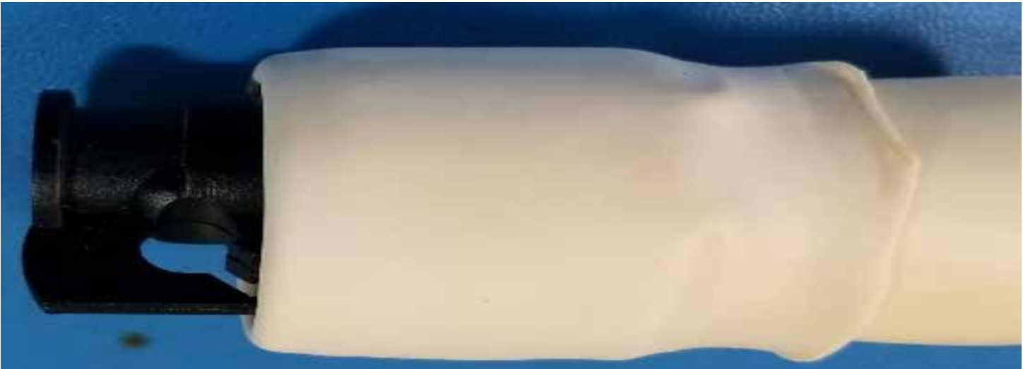
Figure 24 — End of balloon neck pulled back over the retainer ring and valve.
