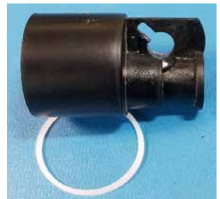
Figure 18 — Recovered valve and retainer ring.
