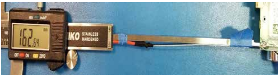
Figure 5 — The optimum antenna length for 433 MHz use is 163 mm, measured from the end of the board.
