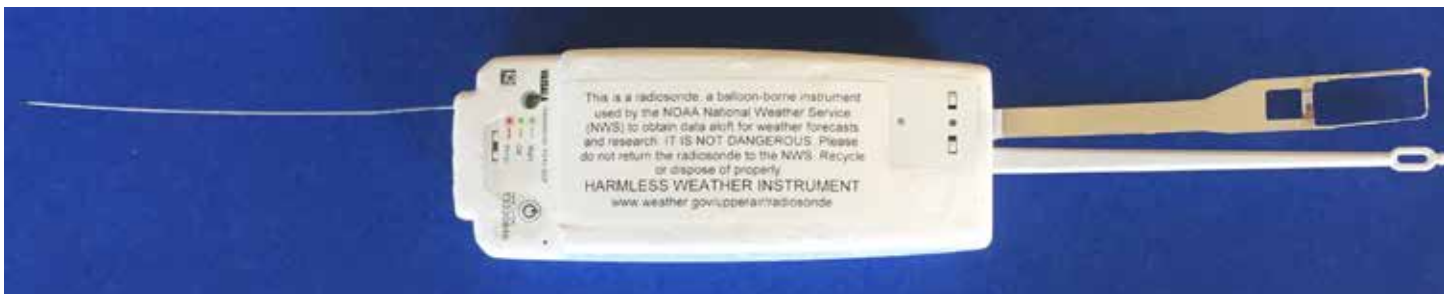
Figure 2 — Recovered Vaisala RS-41 sonde. Note markings: “Please do not return the radiosonde to the NWS” and “HARMLESS WEATHER INSTRUMENT.”
