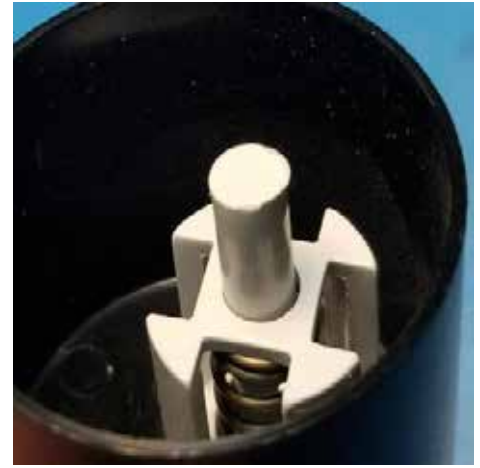
Figure 21 — Internal side of valve, open position.
