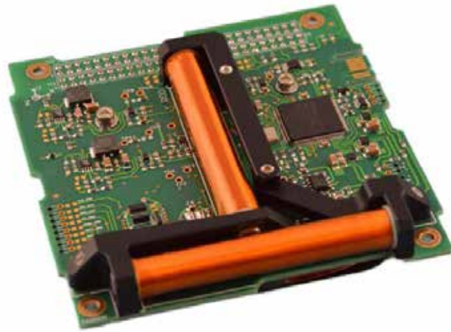
Figure 1 — ISISPACE MagneTorQuer Board as listed on CubeSatShop.com ( www.cubesatshop.com/product/isis-magnetorquer-board/ ).
