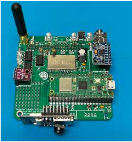
Figure 6 — Development version of CubeSatSim using a Raspberry Pi Pico microcontroller instead of a Pi Zero.
