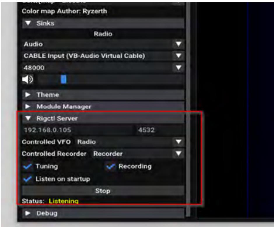
Figure 5 — Rigctl Server on sdr++.
