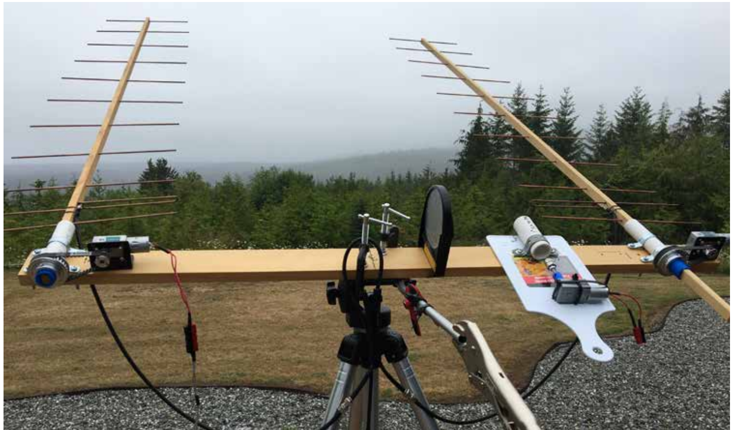
Figure 13 — Two 11 EL Yagi's coax phased with gear motors and remote axial rotation control by VFD.
