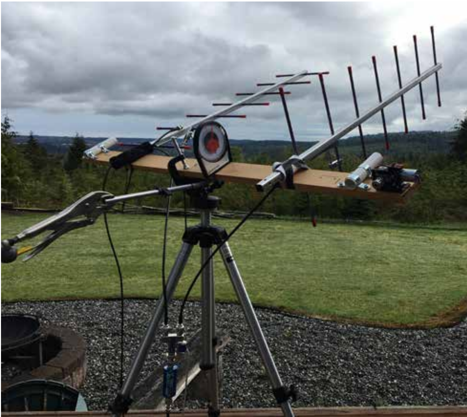
Figure 6 — Two Arrows, remote coax switched for vertical or horizontal.
