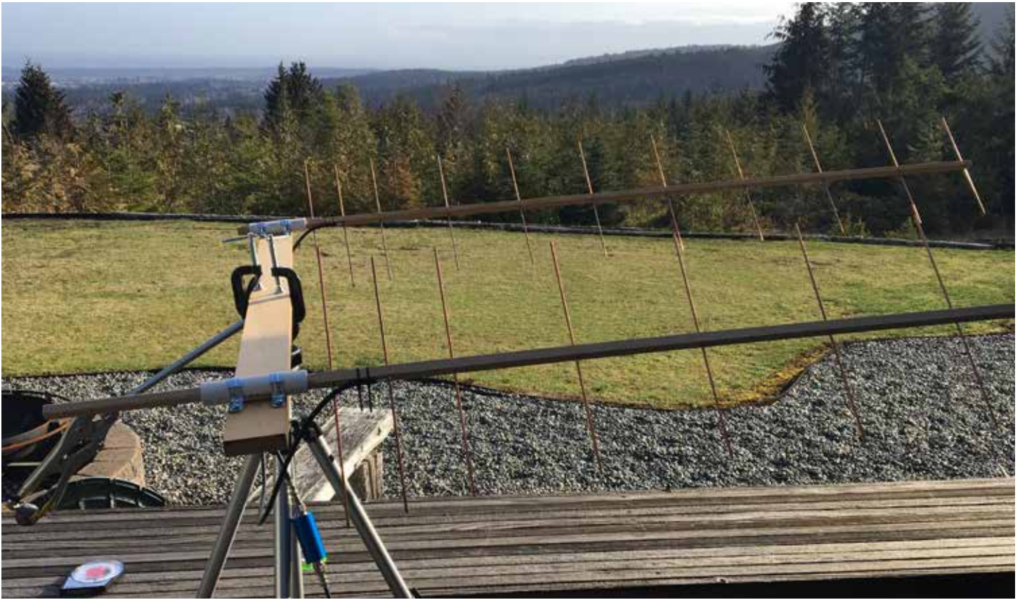
Figure 12 — Two 11 EL Yagi's coax phased and manually rotated for vertical or horizontal or between.
