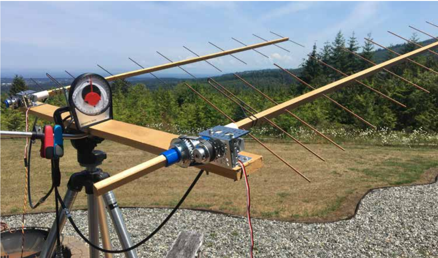
Figure 14 — Two 11 EL Yagi's coax phased with RC Servos and remote axial rotation control by Servo.
