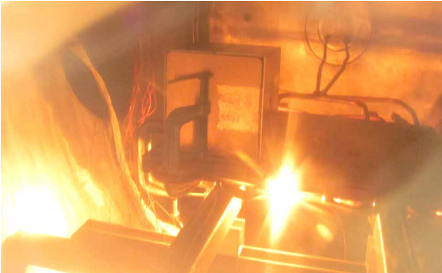
Figure 8 — View inside the chamber during test, illuminated by heater lamp during pulse.
