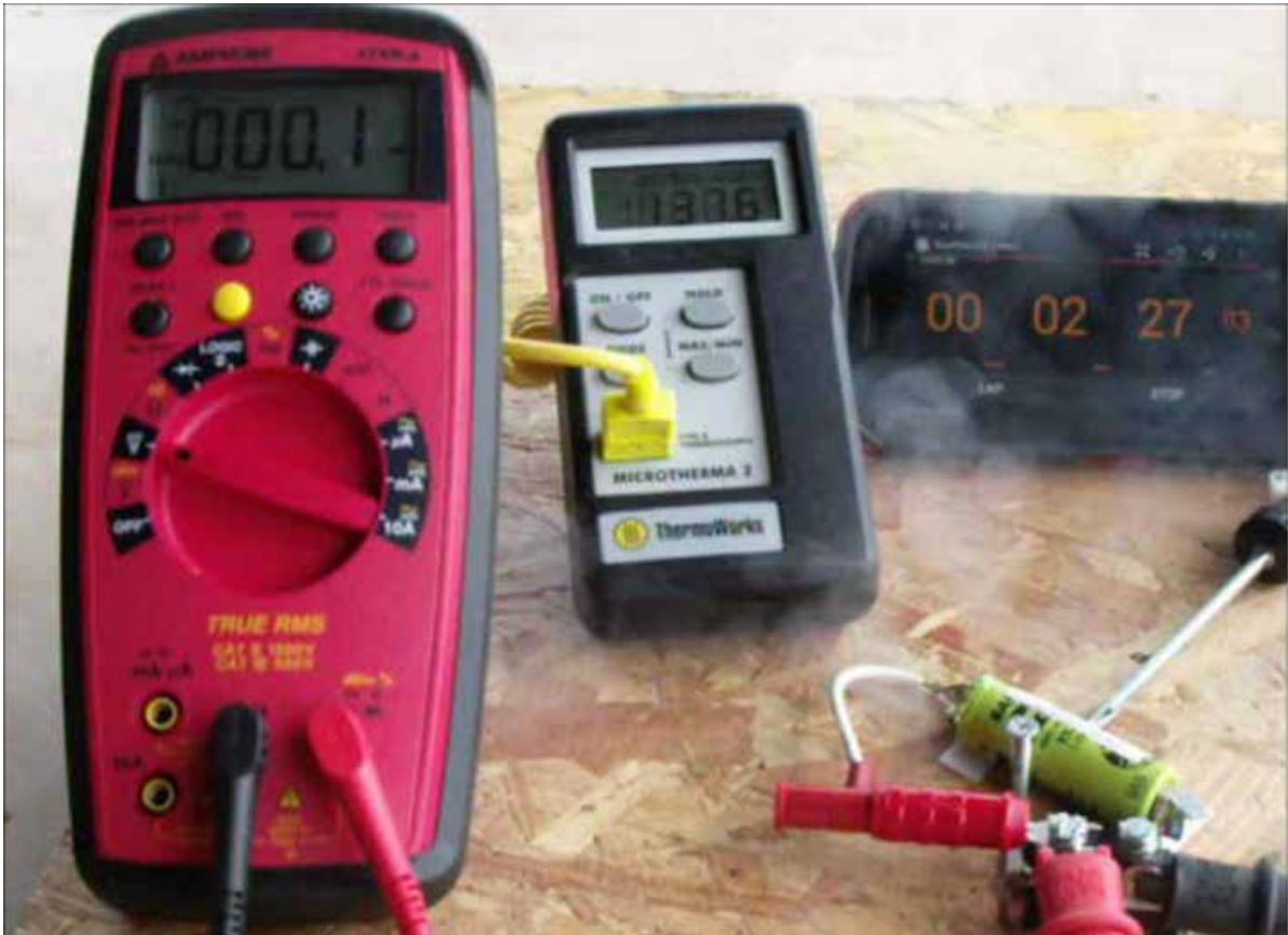
Figure 5 — The venting at 2 minutes 37 seconds is shown here. Recall that the stopwatch is 10 seconds behind the real event time. The venting lasted about 5 seconds.
