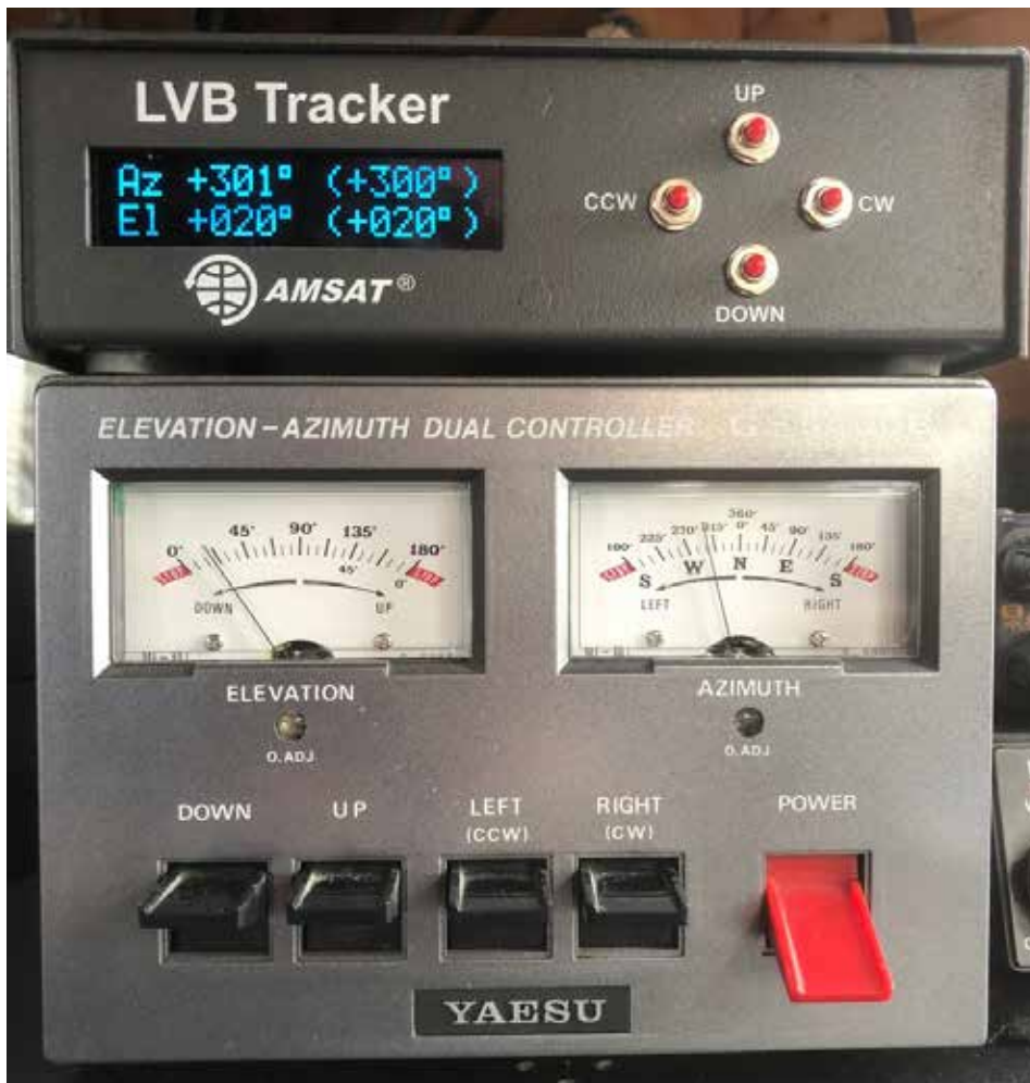
Figure 3 — When connected between your computer and satellite antenna rotator box, a tracking interface, such as the AMSAT LVB Tracker, does a superb job of un-complicating many of the tasks required to use our satellites. While no longer in production, LVB Tracker boxes can still be found on the used market. (Courtesy: Author)
