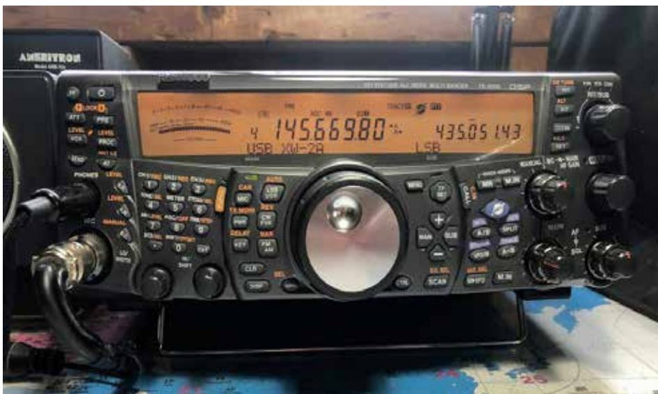
Figure 1 — The author's Kenwood TS-2000S is a 1990s-era, HF/VHF/UHF satellite-capable radio that, while allowing for computer input to compensate for Doppler shifts, still works very well with manual tuning. (Courtesy: Author)
