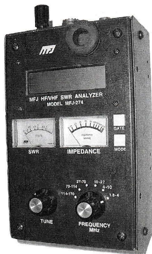
Figure 8.1 — A rubber grommet, higher than the ON/OFF switch on this MFJ antenna analyzer, helps keep it from being accidentally turned on.
