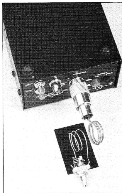
Figure 7.3 — The “grid dip oscillator” probe of Figure 7.2 in use, measuring the resonant frequency of a VHF tuned circuit.
