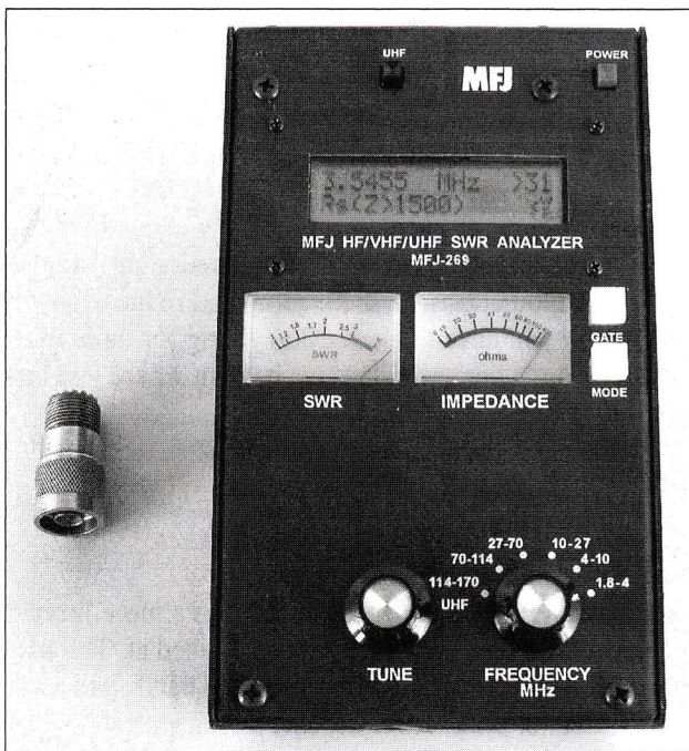
Figure 9.2 — The MFJ-269 antenna analyzer extends the MFJ line into the UHF range and provides considerable flexibility by having external access to its frequency counter.
