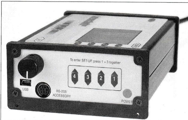
Figure 9.11 — The Timewave AntennaSmith controls are mounted on one side of the unit.
