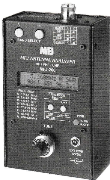
Figure 9.22 — The MFJ-266 antenna analyzer includes many features of the previously discussed MFJ-269 at a lower price and in an entirely, more compact envelope.
