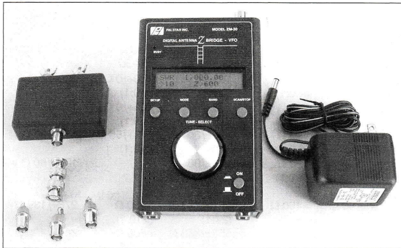
Figure 9.4 — The Palstar ZM-30 offers a lot of advanced features, including reading the sign of the reactance, over the HF range.
