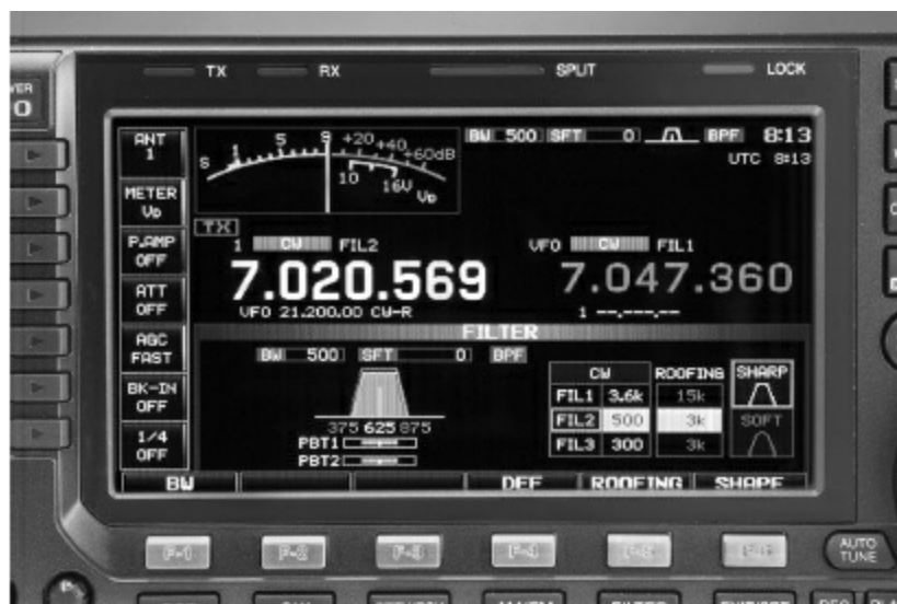
Figure 9.3 — The graphic display on Icom's IC-7600 shows quite a bit of information about filter settings in the lower part of this screen.
