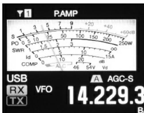
Figure 12.3 — As graphic displays on higher end transceivers such as the Kenwood TS-990S become more sophisticated, manufacturers are able to replicate an a traditional analog S meter in graphic form. As with the analog meter shown in Figure 12.2, this display also monitors a number of parameters on transmit.
