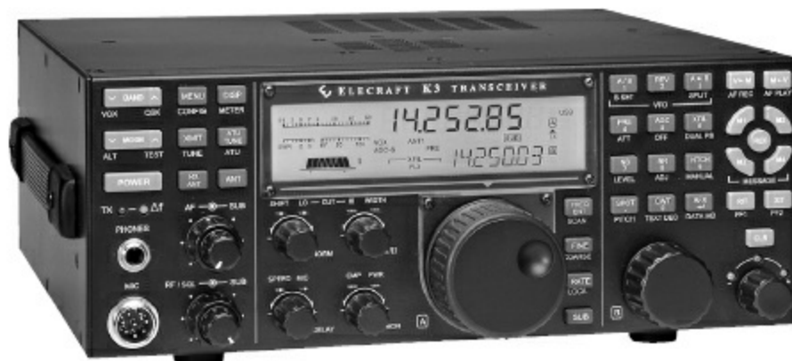
Figure 1.1 — Elecraft's K3 is a current example of a transceiver with coverage from 160 through 6 meters right out of the box.
