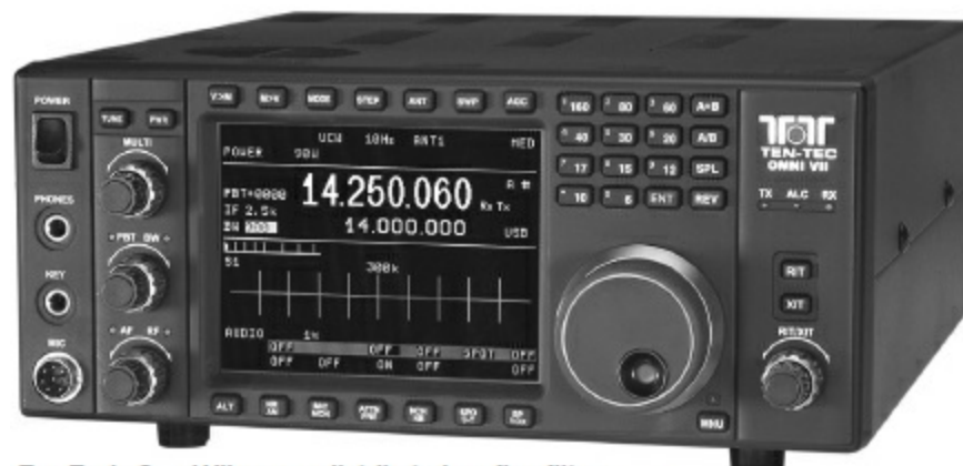
Ten-Tec's Omni VII uses a distributed roofing filter architecture to improve performance. With manufacturing, sales and service in Tennessee, Ten-Tec has a long-standing reputation for excellent customer support.
