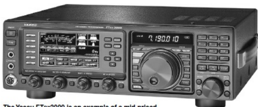
The Yaesu FTdx3000 is an example of a mid-priced transceiver incorporating a colorful TFT display.
