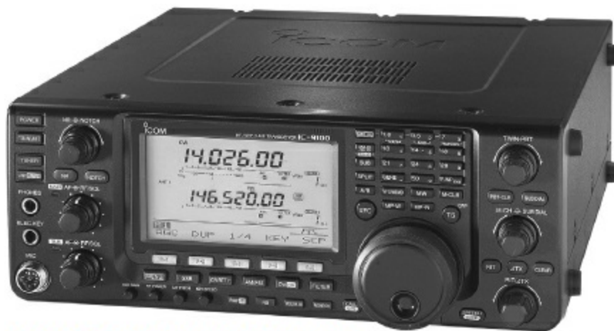
The Icom IC-9100 covers 160 through 2 meters, plus 70 cm with an option for 23 cm (1.2 GHz) operation. It uses a large, highly readable LCD screen to clearly display operating frequency and other information.
