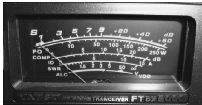
Figure 12.2 — In this Yaesu FTDX1200 transceiver, the analog S meter is also used on transmit to measure compression, ALC, power output, drain current, drain voltage and SWR.
