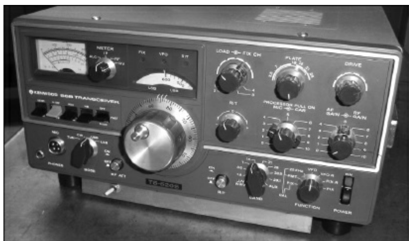
The classic Kenwood TS-520S from 1978 sold for about $2400 in today's dollars and lacked many of the features we take for granted in a modern HF transceiver.
