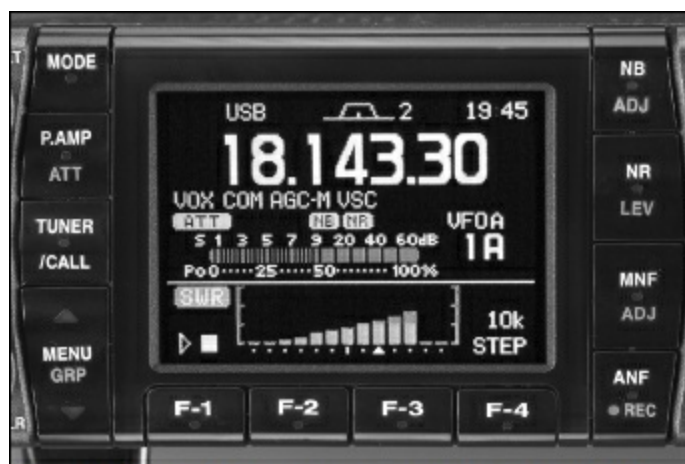
Figure 12.4 — Smaller transceivers, such as the Icom IC-7000, incorporate a bar graph S meter in the display.
