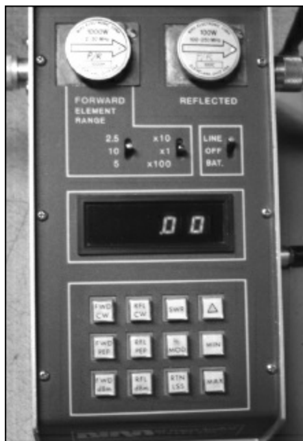
Figure 13.1 — A Bird 4391 power meter used for measuring RF power output.
