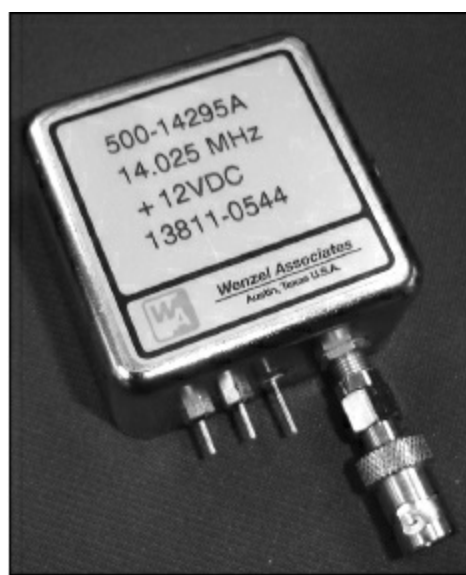
Figure 5.2 — Wenzel test oscillator used for reciprocal mixing test.
