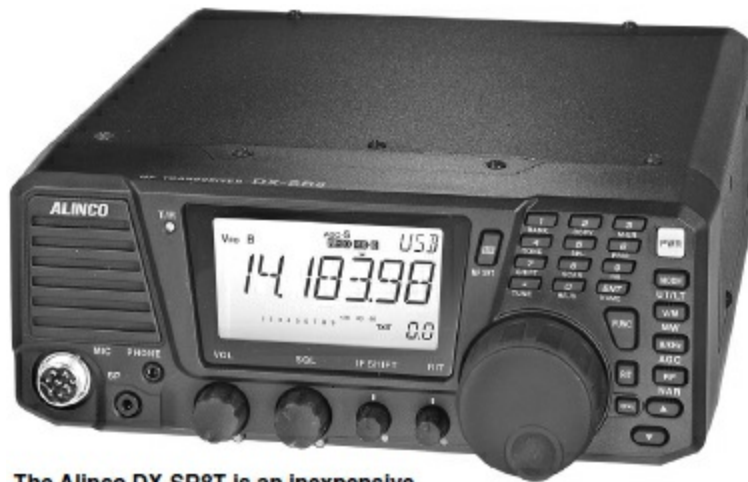
The Alinco DX-SR8T is an inexpensive 160-10 meter transceiver. Its front panel is detachable for easier installation in a mobile station.
