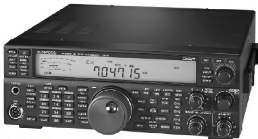
The simple LCD on Kenwood's TS-590S includes bar graph metering functions for transmit and receive, as well as a number of indicators showing the status of various transceiver settings.
