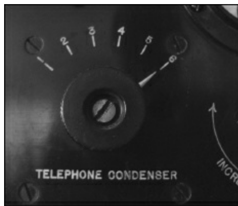
Figure 9.2 — A close up of the IP-501 shows an early attempt of filtering out high-pitched audio tones with the control labeled, “Telephone Condenser.”
