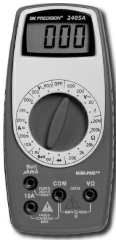
Figure 6.5 — A B&K Precision model 2405A DMM. This is a basic 2.5 digit display, manual ranging, tool-box type model priced at about $32 (as of mid-2015) that does almost everything that a VOM can do. [Photo courtesy of B&K Precision]
