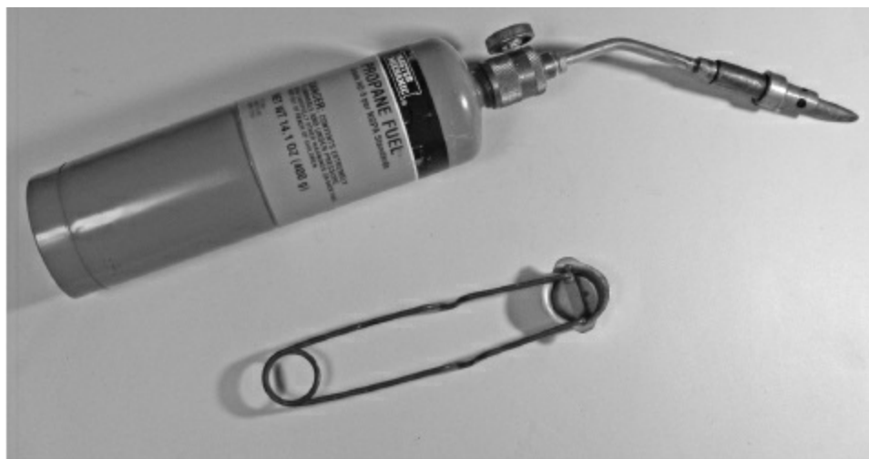
Figure 3.5 — A plumber's type of portable propane torch with a chisel-type add-on head designed for heavy-duty soldering. The igniter is used to start the flame with the tip removed and then the tip can be attached carefully with pliers.
