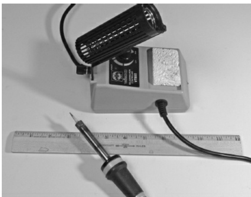
Figure 3.3 — An inexpensive soldering station. The soldering station provides continuous control of iron temperature through the knob included in the base. While precise control is not provided by this arrangement, it does allow easy adjustment for different conditions.
