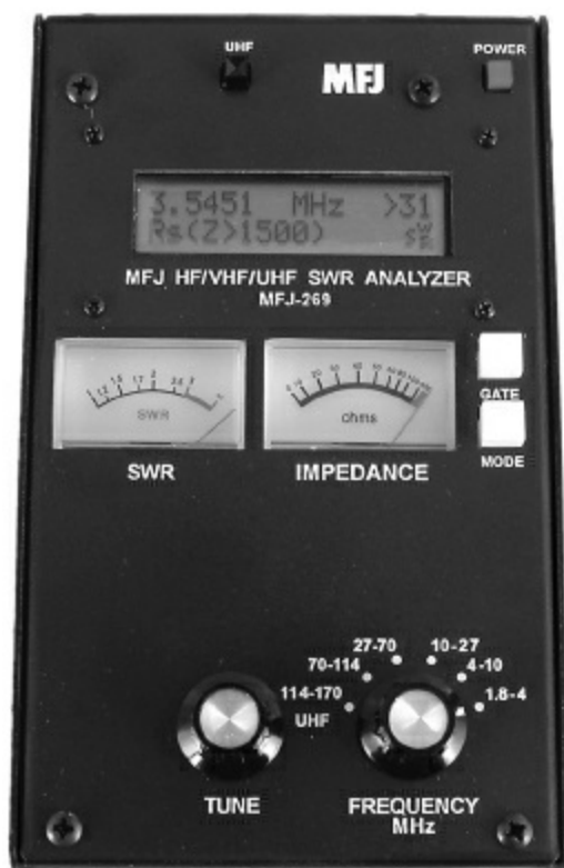
Figure 7.8 — An MFJ-269 antenna analyzer. In addition to its antenna analysis functions, this unit is particularly useful because the frequency counter can be accessed independently.
