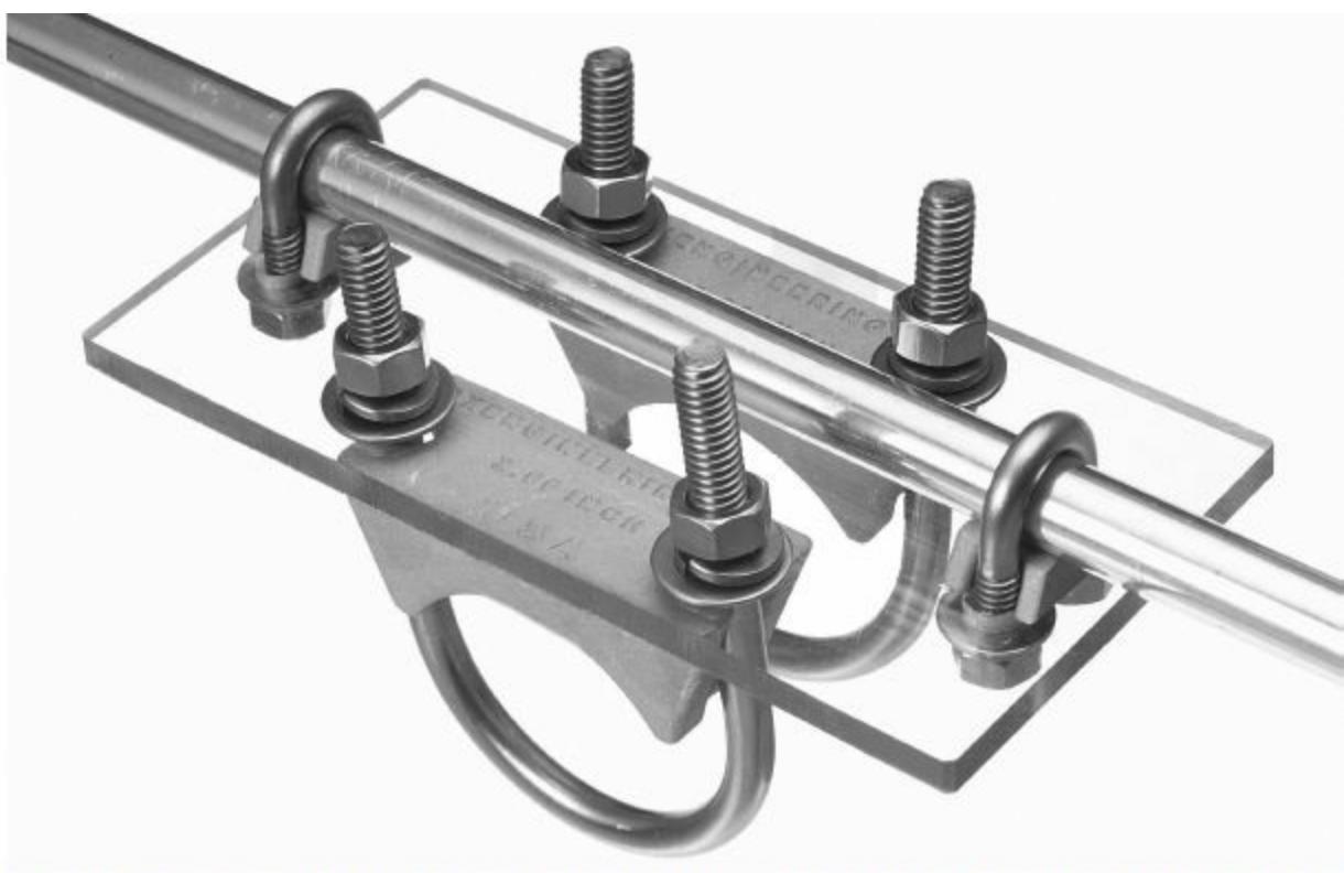
Figure 5.6 — The author made use of DX Engineering ( www.dxengineering.com ) stainless steel saddle clamps to hold the elements of his 6 meter coupled-resonator Yagi to the boom via a polycarbonate insulating mounting plate.
