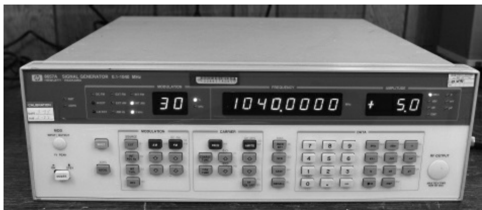
Figure 7.16 — The HP-8657A signal generator covers 100 kHz to 1040 MHz and includes a precision output level adjustable from +17 to -143.5 dBm. [Photo by Dustan Dennington / DennLec.com]
