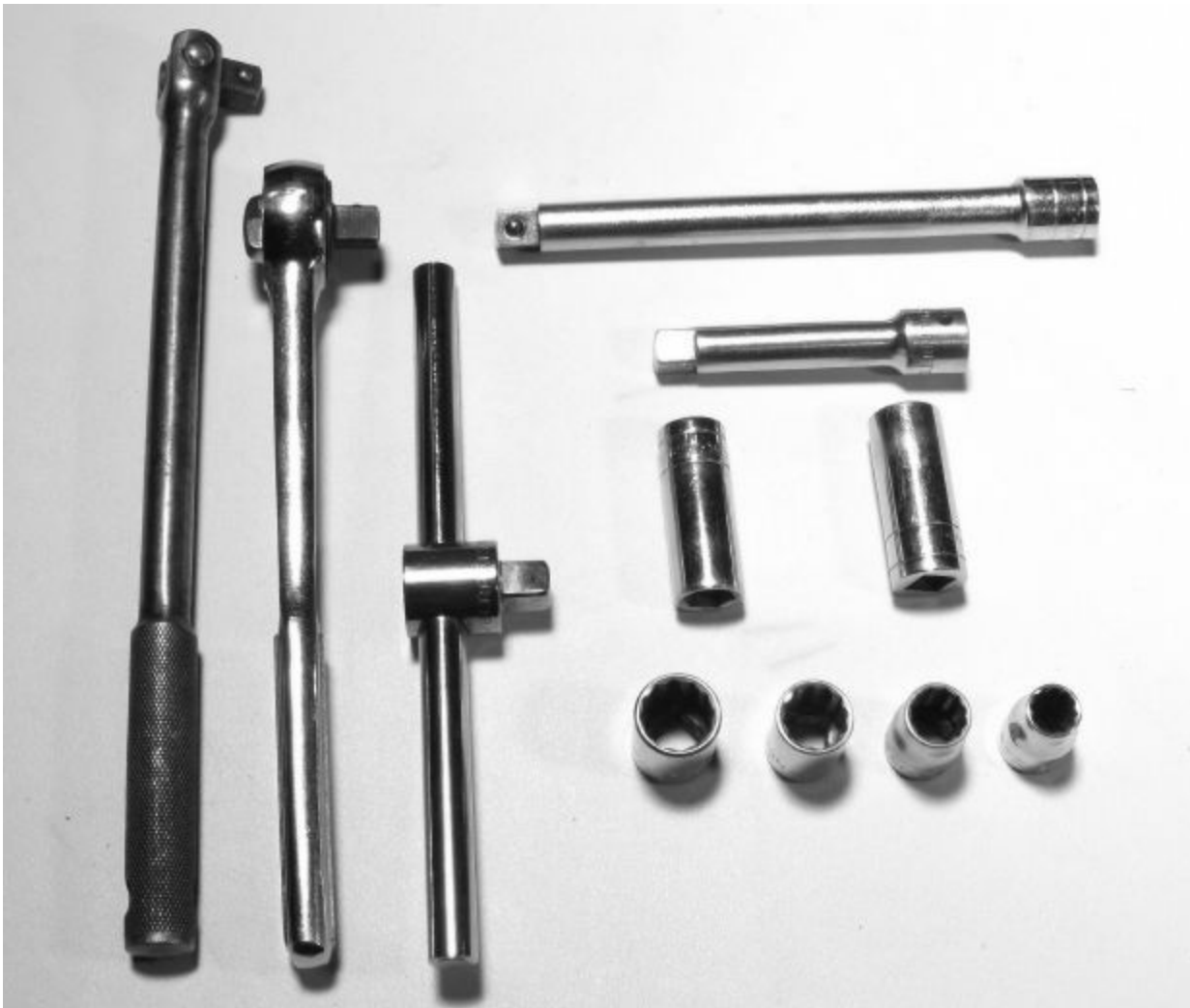
Figure 5.7 — Selection of \frac{3}{8} inch drive socket wrenches and extension bars, with ratchet, bar, and T-handles. While \frac{5}{16} , \frac{3}{8} , \frac{7}{16} , \frac{1}{2} , and \frac{9}{16} inch sizes are most frequently needed, it is often more economical to buy a packaged set than individual wrenches. The extra-long (“deep”) sockets are handy for clamps with long threaded sections.
