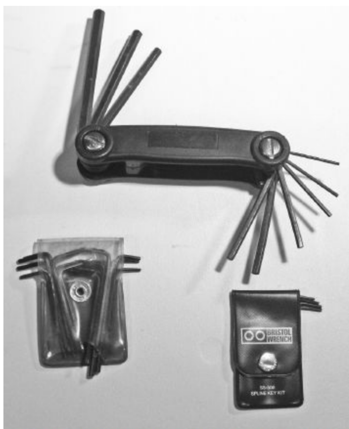
Figure 2.6 — Tools for use with screws that have hex socket heads. The tools on top and the set on the lower left are the popular Allen head wrenches, frequently used in set screws. The tools on the lower right are Bristol spline wrenches, superficially similar in appearance to Allen wrenches, but not compatible.
