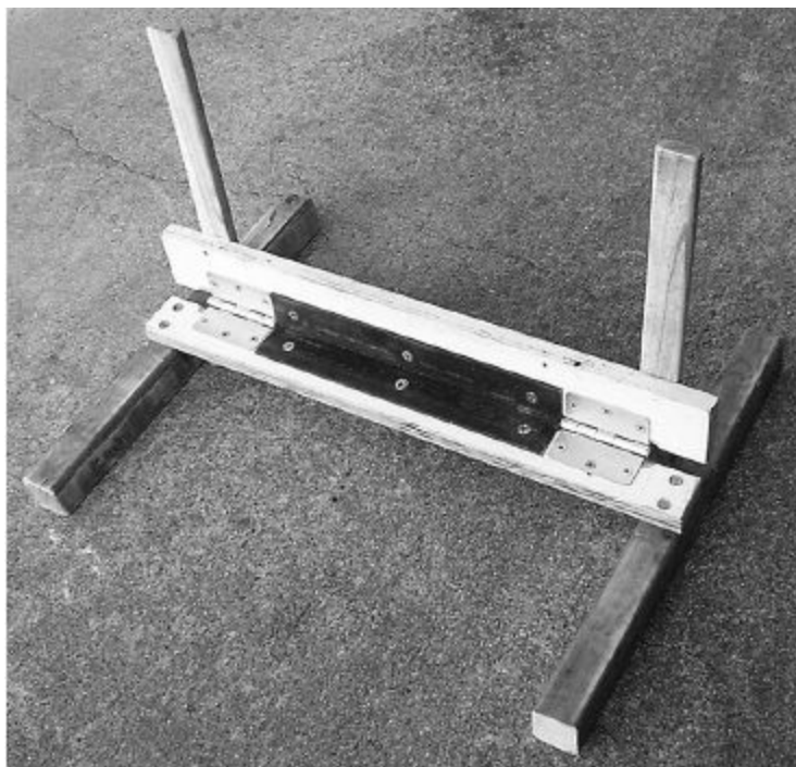
Figure 9.6 — A home-made metal bending brake made from wood, some door hinges and metal mending plates. This can be used to fabricate bent aluminum chassis boxes, but read reference 3 before you start.
