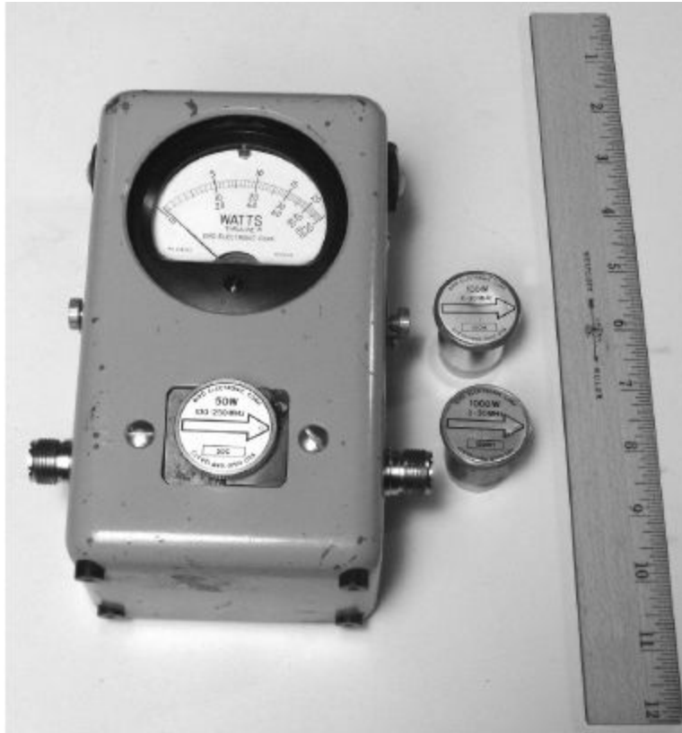
Figure 6.9 — The author's Bird model 43 directional wattmeter. Different elements or "slugs" are inserted into the front, depending on the frequency range and power level being measured. The slug can be rotated to change the direction of power measurement.
