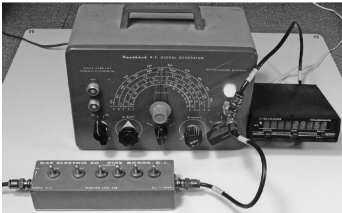
Figure 7.13 — A signal generator with limited capability can be improved significantly with outboard accessories that are useful in many other functions — a frequency counter and a step-attenuator (available from Elecraft and MFJ, in addition to commercial surplus). While the signal generator won't provide a calibrated output level, the known change in level provided by the attenuator can be used to measure improvement in gain.
