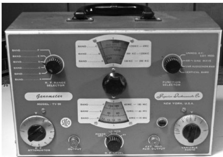
Figure 7.12 — A somewhat more capable signal generator from the same period with added touches intended to facilitate analog TV servicing. This is a Superior Instruments TV-50 signal generator that includes modulation designed to result in horizontal or vertical bars on an analog TV screen, as well as cross hatch and dot patterns.
