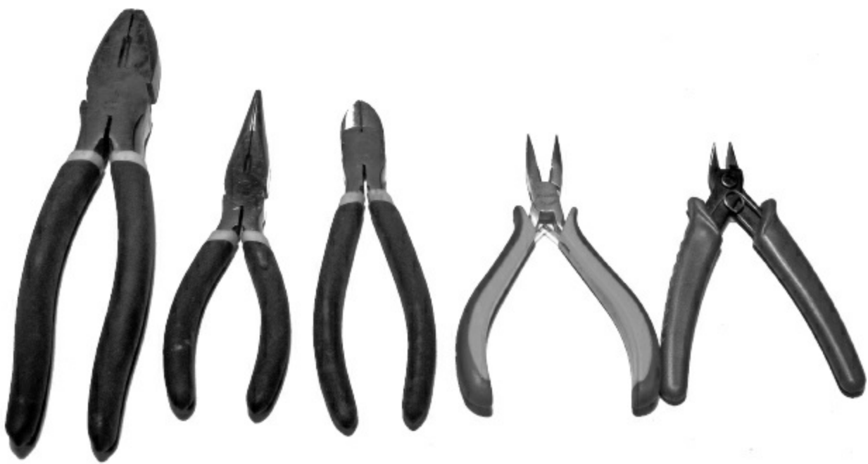
Figure 5.1 — Comparison of tools for making wire antennas with those for electronic component work. The larger ones on the left are for the larger size antenna wire.
