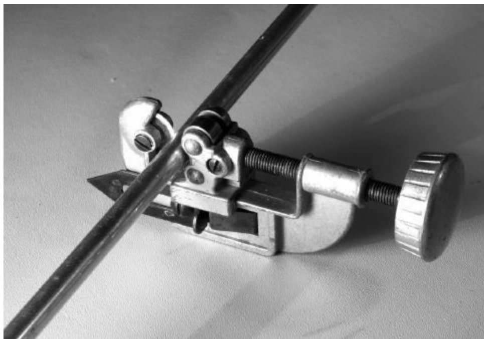
Figure 5.5 — A simple hardware store tubing cutter easily makes smooth, square cuts from pieces of aluminum or copper tubing. The reaming blade, shown extended in this photo, allows removal of the ridge formed inside the cut ends — important to remove only if smaller tubing must telescope into the end.
