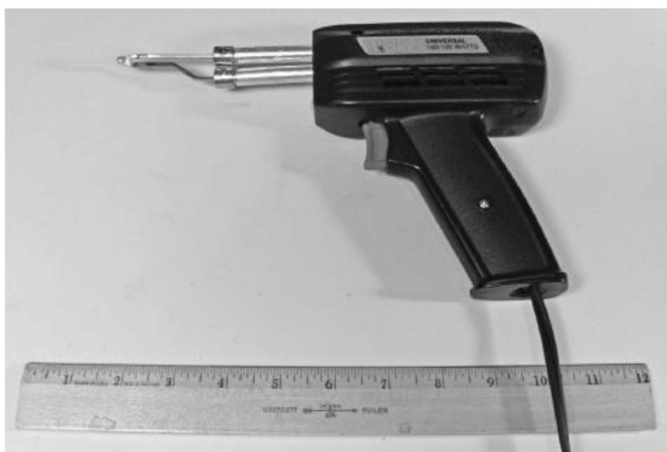
Figure 3.1 — A Weller 100/140 W “instant-heat” resistive soldering gun. The trigger switch has two positions, the first for 100 W and the second for 140 W. The “instant” is somewhat optimistic, but in comparison to earlier soldering irons that took perhaps 15 minutes to come to temperature, it was a meaningful term.
