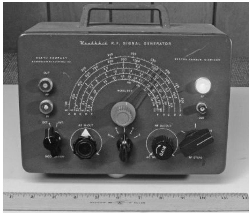
Figure 7.11 — A Heathkit SG-8 RF signal generator from the 1950s designed for broadcast and shortwave radio service. This unit covers from 200 kHz through 111 MHz on fundamental frequencies. Internal and external AM modulation is supported, along with an adjustable (but not calibrated) RF output. The scratches and mixed knob style are the consequences of many years of hard service.
