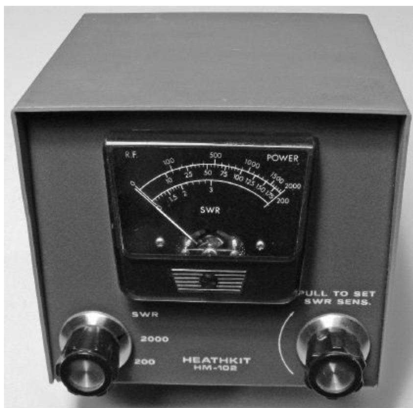
Figure 6.10 — This 1970s vintage Heathkit HM-102 power meter can measure forward power as well as SWR over the HF range. It has a remote sensor that can be inserted into the antenna feed system away from the operating position.
