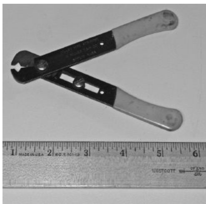
Figure 3.6 — A classic “Miller” wire stripping tool. This sample has been in the author’s family for about 60 years and is still going strong. The original manufacturer, K. Miller T & M Company from West Springfield, Massachusetts, is no longer in the picture, but similar tools are being made by others. Some offer advanced features, such as a return spring and a wire size selector.
