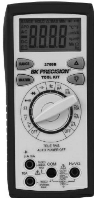
Figure 6.6 — A B&K Precision model 2709B DMM. This unit is auto-ranging, measures dc voltage to 1000 V, true RMS ac voltage to 750 V, capacitance, frequency to 66 MHz, and checks diodes. It has a 3.75 digit display and lists for $105 (as of mid-2015). [Photo courtesy of B&K Precision]
