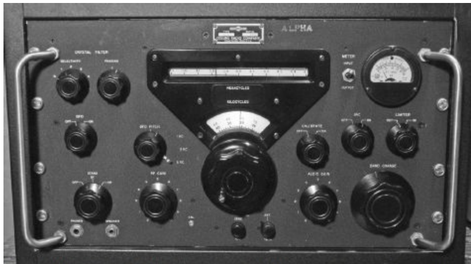
Figure 7.17 — The Collins 51J4 receiver from the 1950s can read frequency to less than 1 kHz — about as good as the analog technology of its day, and better than almost all other contemporary receivers. Most current HF transceivers can read frequency to 1 Hz, three orders of magnitude higher resolution.
