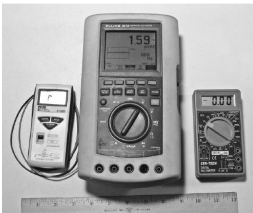
Figure 6.4 — Representative digital multimeters (DMMs). The larger Fluke model is a professional quality unit, while the smaller Ideal unit on the left is typical of an autoranging “toolbox” DMM.
