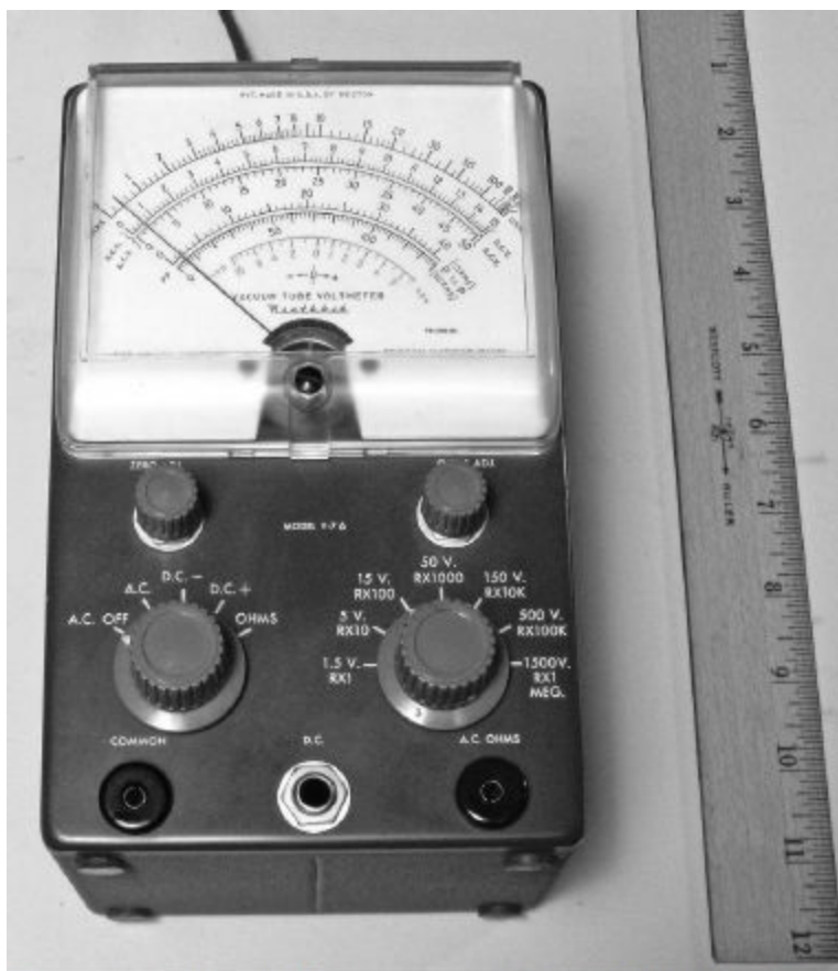
Figure 6.3 — A Heathkit V-7A vacuum-tube voltmeter (VTVM) from the 1950s. This solved the VOM circuit loading problem by offering an input impedance of 11 M \Omega .
