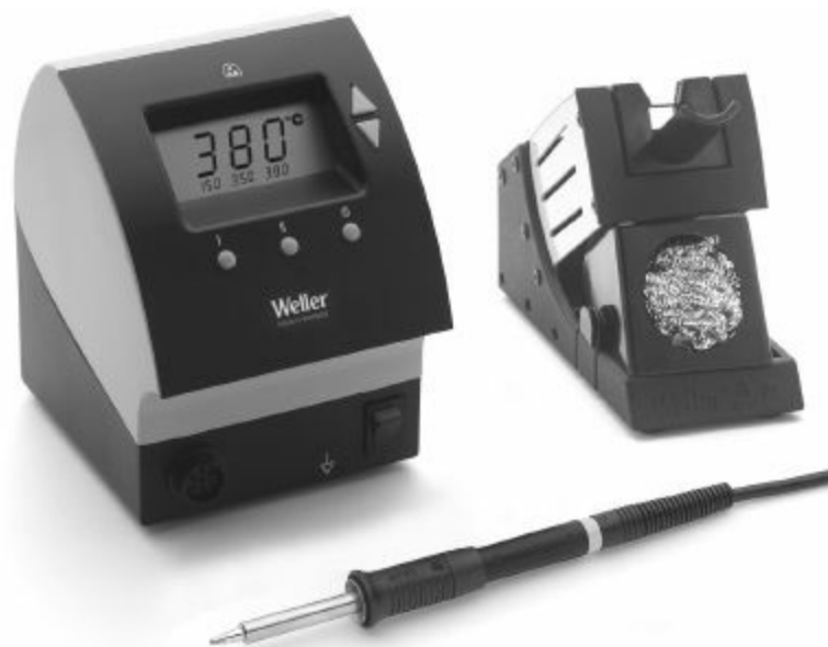
Figure 3.4 — The Weller WD-1000 temperature controlled soldering station. This unit automatically regulates the iron tip temperature to the desired setting. The settings can be adjusted manually using the switches on the right side of the control, or three temperatures can be programmed in and accessed with a single push of the appropriate button beneath the display. [Photo courtesy of Apex Tool Group, LLC]
