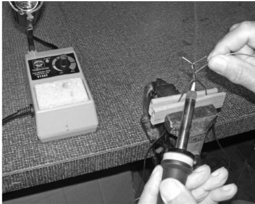
Figure 3.8 — The author is soldering a pair of bare copper wires. Note that the wires are held in place by a small machinist's vise. Two strips of wood provide thermal insulation from the jaws so the heat will not be drawn away. The hot iron is applied to both wires from beneath to allow the heat to rise to the soldering region, while the solder is applied to the wire until it flows smoothly.
