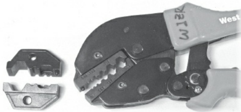
Figure 4.5 — The crimp tool of Figure 4.3 with dies changed to support crimping coax connectors. Note that there are multiple dies required to deal with various coax connector types.
