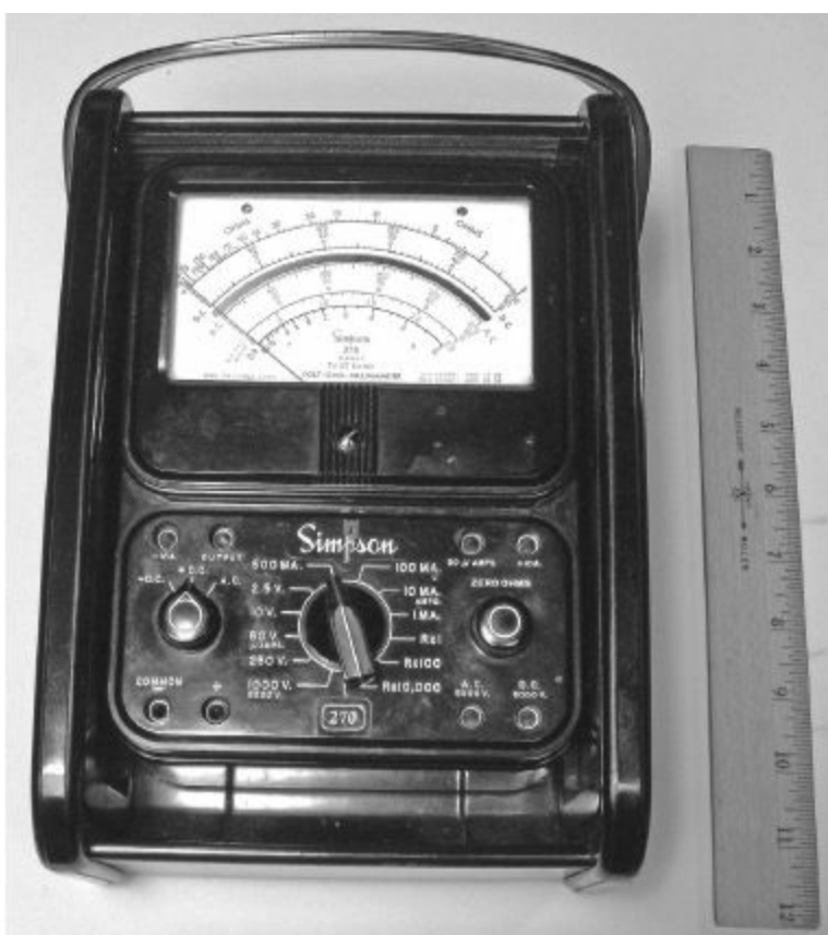
Figure 6.1 — The author's 50-year-old Simpson 270RT VOM is representative of the basic volt-ohm-milliammeter (VOM) functionality.
