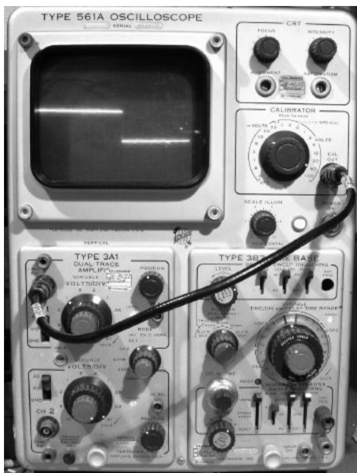
Figure 7.22 — The author's vintage Tektronix 561A dual-trace oscilloscope. This is typical of the many scopes of its era and includes the capability to accept plug-in drawers to change both the horizontal time base and vertical input ranges. The delayed sweep function allows detailed examination of a portion of a waveform.
