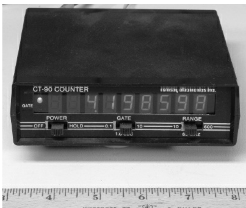
Figure 7.18 — An inexpensive frequency counter. This one is a Ramsey Electronics CT-90 from 1998.
