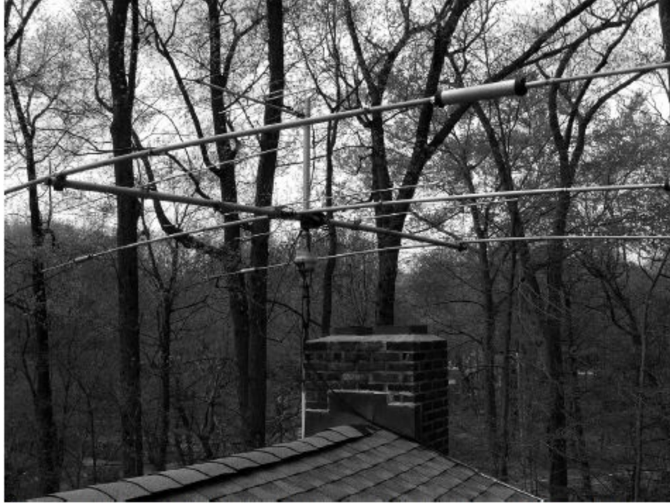
The author's HF triband Yagi with coupled-resonator 6 meter add-on. The tribander is a commercial model, the 6 meter portion homemade. Similar tools were required to assemble each.
