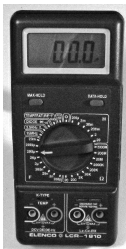
Figure 6.8 — A special purpose DMM designed to measure the value of resistors, capacitors and inductors.
