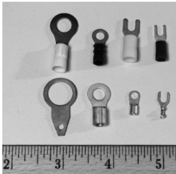
Figure 4.8 — Eye or ring terminals (left) and spade terminals (right) are a convenient way to make a secure connection to a chassis, barrier strip, or any other connection under the head of a screw. The top row shows the insulated type, while the bottom row shows the uninsulated version. While eye or ring terminals are more secure, spade terminals can be removed without completely removing the screw or bolt.
