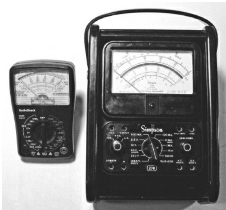
Figure 6.2 — A RadioShack portable VOM shown next to the Simpson 270RT from Figure 6.1.
