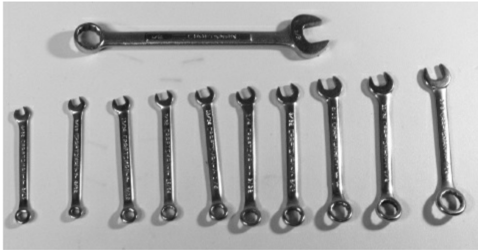
Figure 2.8 — These smaller combination wrenches, often marketed in a set as ignition wrenches , are frequently a better choice than their larger siblings for radio work. A typical 3/8 inch combination wrench is shown for comparison.
