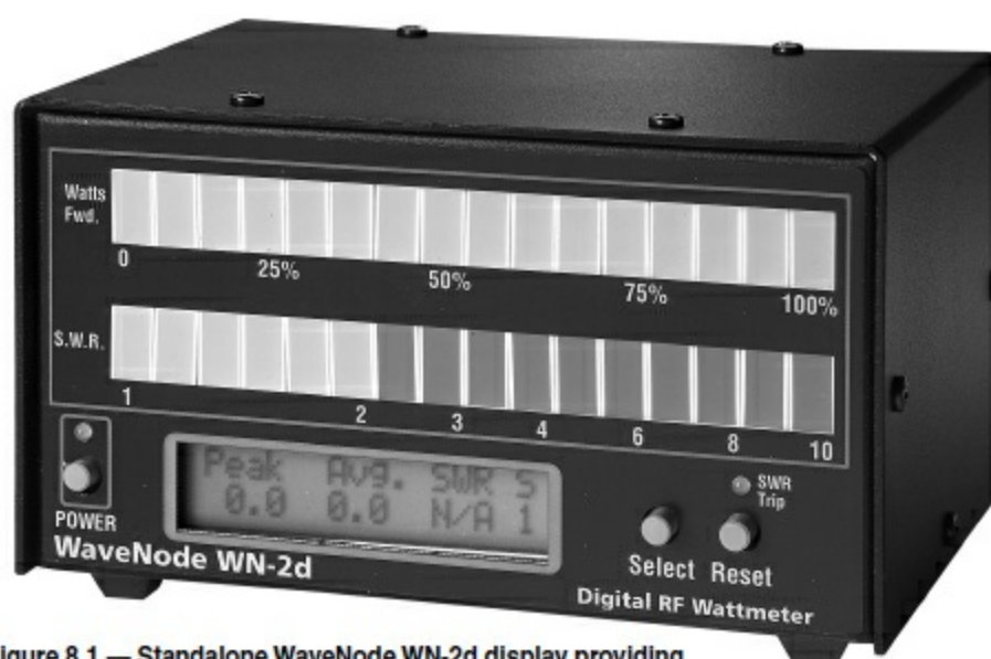
Figure 8.1 — Standalone WaveNode WN-2d display providing numerical indication of peak power, average power, and SWR for any of up to four remote power sensors.
