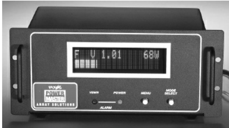
Figure 6.12 — Array Solutions PowerMaster ( www.arrayolutions.com ) power meter. This measurement system can function as a standalone instrument with its built-in display, or provide output to a connected PC, as shown in Figure 6.13.
