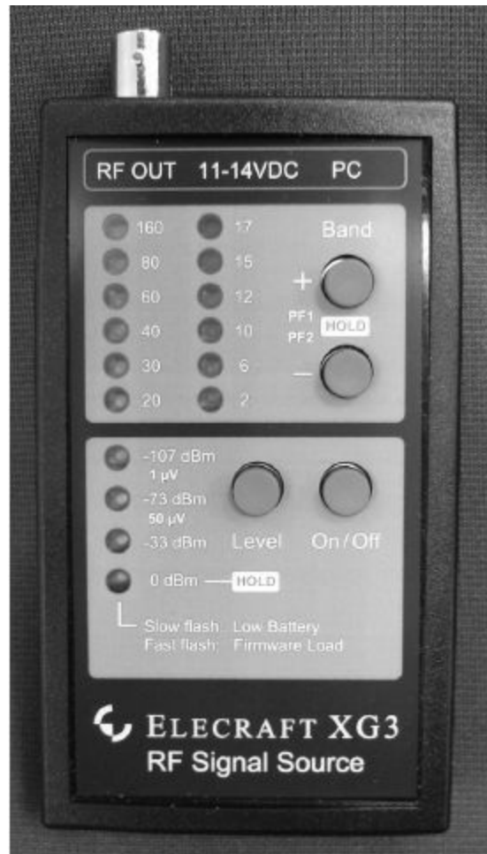
Figure 7.10 — The Elecraft XG-3 RF Signal Source. This generator provides synthesized RF signals from 1 to 200 MHz at four selectable output levels, 0 dBm, -33 dBm (40 dB over S-9), -73 dBm (S-9), and -107 dBm (1 \mu V).
