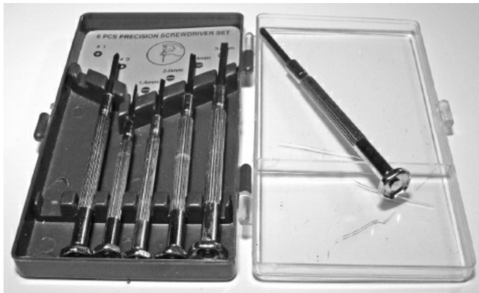
Figure 2.5 — A set of jeweler's screwdrivers. These can be handy for many tasks, but check for quality — all are not created equal.
