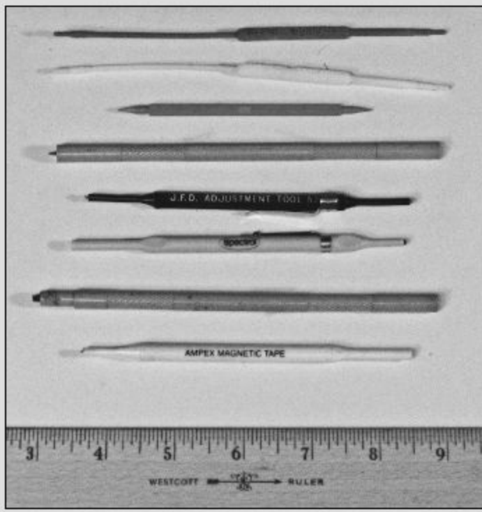
Figure D — Selection of alignment tools from the author's tool box. Note that there are both hex and slotted types. The slotted tools include ones with both protruding and recessed bits. Screwdrivers should be avoided for this task to eliminate tuning changes from the metal shanks as well as a risk of shorting a trimmer to the chassis.
