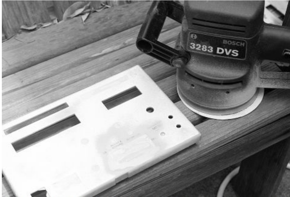
Figure 1.4 — Here Wayne Yoshida, KH6WZ, uses a sander to remove excess paint and auto body filler from a reclaimed test instrument panel that will turn into the front panel of a piece of amateur station equipment. [Wayne Yoshida, KH6WZ, photo]
