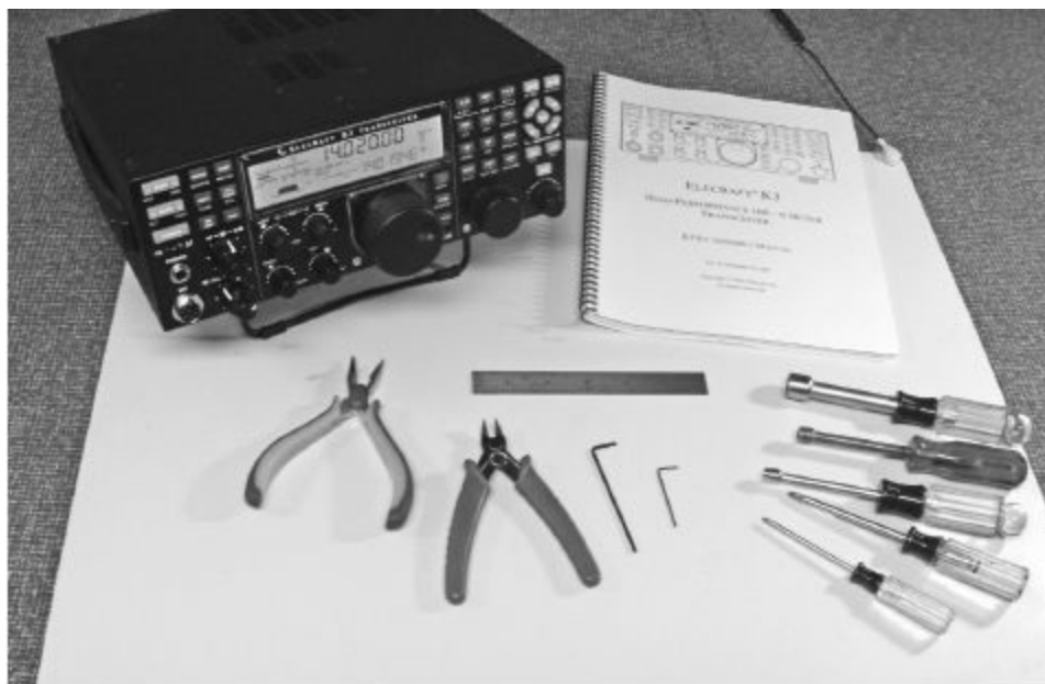
Figure 2.1 — Tools required for assembly of the Elecraft K3, all sitting on the table where the author successfully constructed his K3. The tools, K3, and assembly manual are shown on the recommended electrostatic discharge mat (see text).
