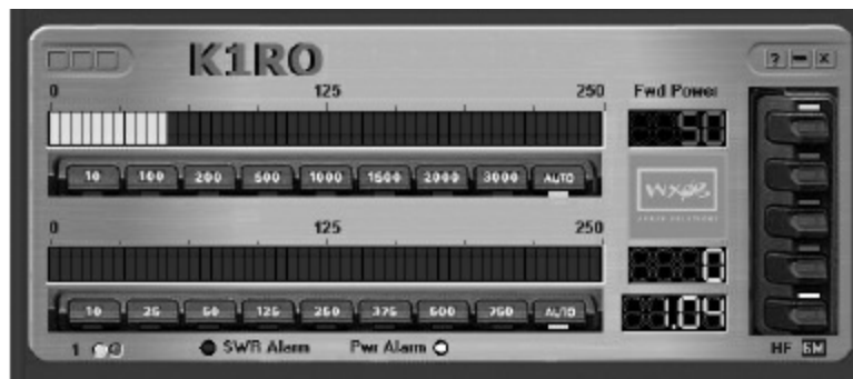
Figure 6.13 — The PowerMaster can display measured data and wattmeter controls on a computer screen, and a miniature version of the display can be monitored while running other applications such as logging software.
