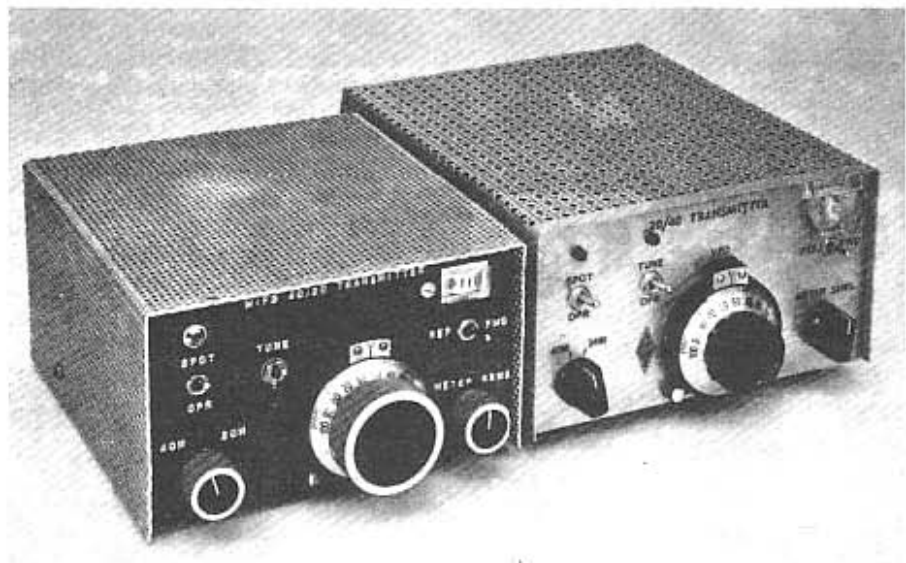
Two versions of the 7- and 14-MHz cw transmitter are shown here. At the left is the W1FB prototype. On the right is a model built by WA0UZO. Both units are small and lightweight.
