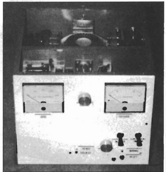
Figure 1—This table-top 2-meter power amplifier uses a quick-warm-up tube, a real plus when the band suddenly opens for DX and you want to join in.
