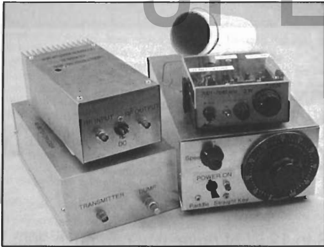
Figure 2—The components of the Class-E amplifier station. Clockwise from bottom left: the diplexer, amplifier, resonant speaker, NorCal 40A and keyed power supply. The latter houses the keyer and a pulse-stretching and shaping circuit.
