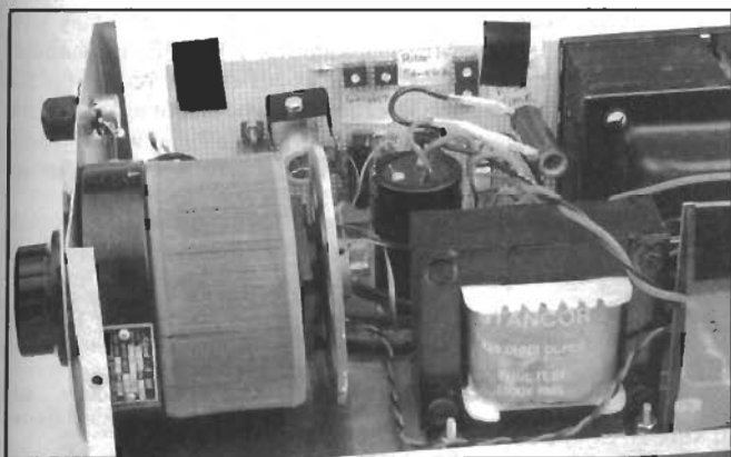
Figure 12—The keyed power supply with the cover removed, viewed from the side. T1 is mounted on the back plate, along with the fuse and connectors for the dc output, a keying line to the NorCal 40A and the ac line input. The TUNE switch keys the amplifier for testing. The variable autotransformer is on the left, mounted to the front panel. In the center foreground, mounted to the base plate, is L1, the 25-mH choke. Mylar sheets are taped to the perboards for electrical isolation. The large components are attached directly to the box. The IRFP340 is mounted on the bottom of the box using a Berquist K10-104 Kapton insulating pad, #6-32 screw and a torque of 10 inch-pounds. The other shaping circuit components are mounted on perboard. Layout is not critical.
