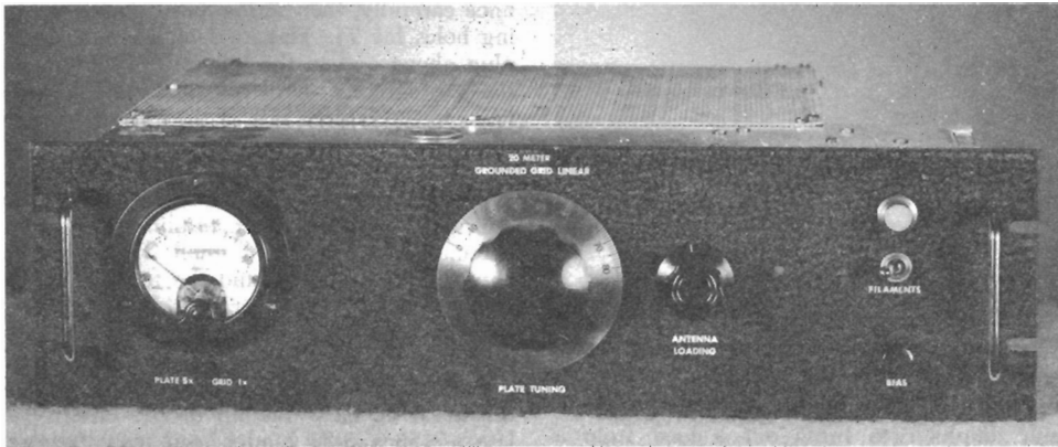
All amplifier units have the same panel design. This unit is the one used for 20 meters. Tuning and loading controls are at the center. The small knob in the lower right-hand corner is for adjusting bias.
