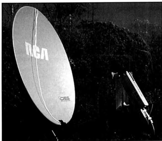
Fig 9—Offset dish receiving sun noise. Feed horn shadow at edge of dish demonstrates minimal aperture blockage by offset feed.
