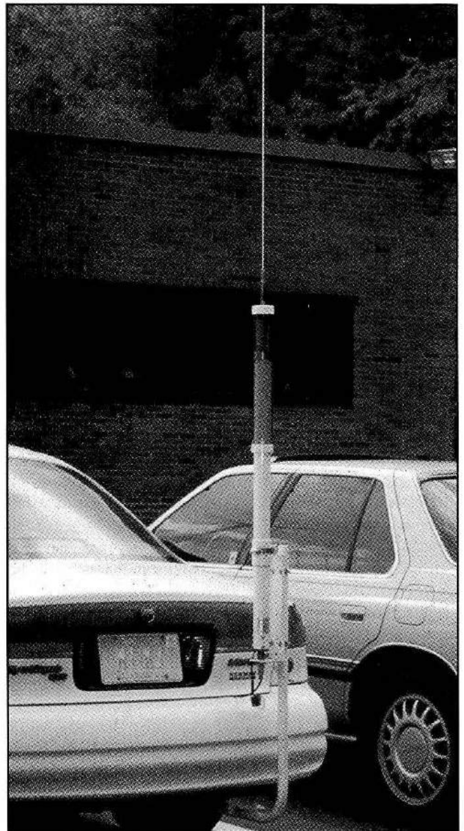
Fig 3-3—A pipe, bar or tow hitch fastened to the undercarriage can make an excellent mount for a large HF antenna.
