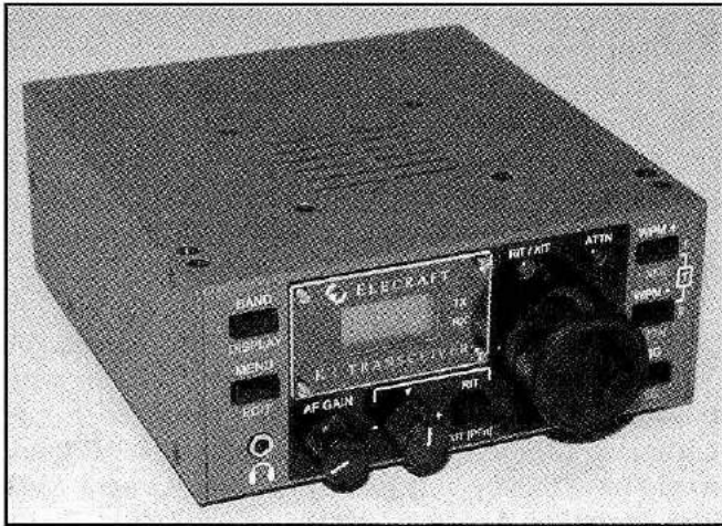
Fig 2-13 —The Elecraft K1 transceiver is one popular transceiver kit. There are several others to choose from as well.
