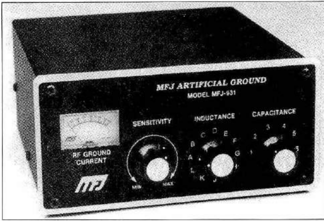
Figure 5-1—The MFJ-931 Artificial RF Ground can help solve “RF in the shack” problems.
