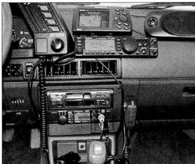
Fig 3-1 —Here the remote head is mounted on the dashboard within easy reach of the driver. Note the 2-meter rig mounted below the car stereo. Dressing the cables so as not to snag or get in the way is another safety consideration.
