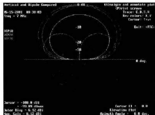
Fig 1-16 —This drawing shows how the vertical compares to horizontal dipoles at different heights.
