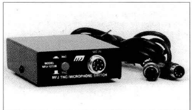
Fig 2-5—The MFJ-1272B switches the microphone input of your FM transceiver between your microphone and packet TNC.
