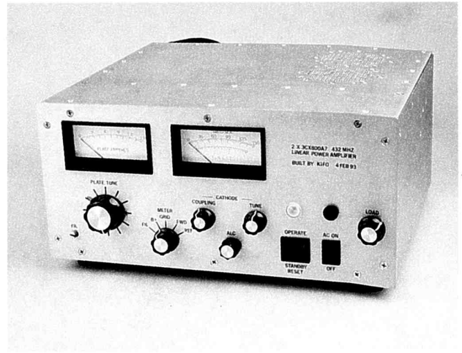
A pair of 3CX800A7 tubes provides a cost-effective means of producing the legal limit on 70 cm.
