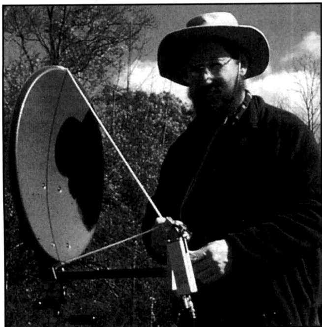
Fig 4—Locating feed point for offset dish using calculated string lengths.
