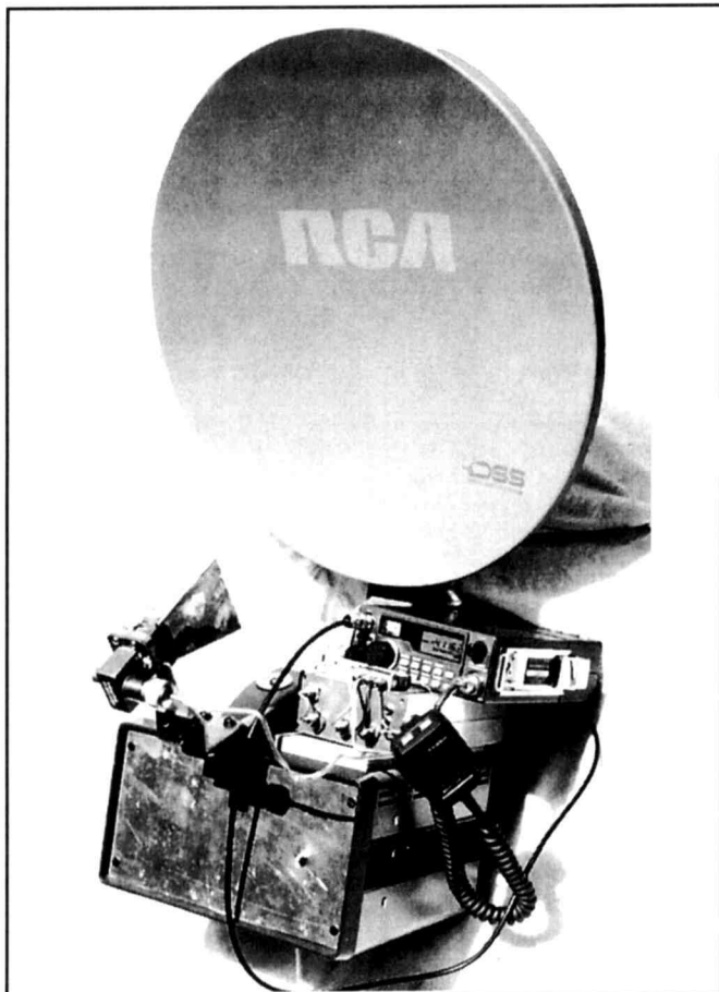
Figure 1—Dual-band rover system for 5760 and 10368 MHz.
