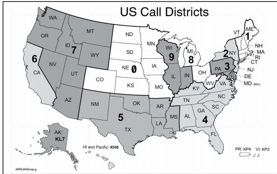
Figure 2— There are 10 US call districts or areas. Hawaii and all Pacific possessions are part of the sixth call area and Alaska is part of the seventh. Puerto Rico and the US Virgin Islands are part of the fourth district.
