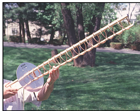
Most communication with space, both manned shuttles and unmanned satellites, uses VHF, UHF or microwave frequencies. This homebrewed antenna was designed to be used for a new satellite called Phase 3D .
