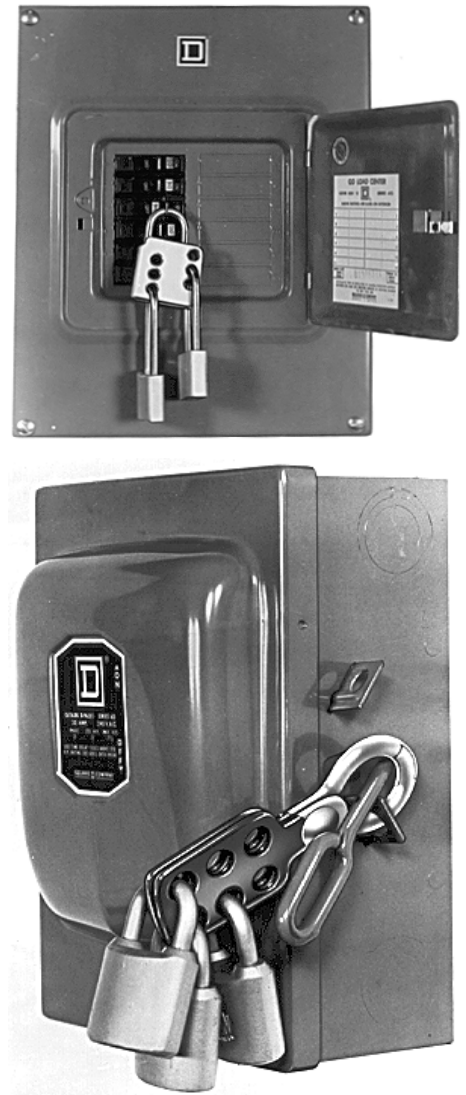
Fig 9.2—If the switch box feeding power to your shack is equipped with a lock-out hole, use it. With a lock through the hole on the box, the power cannot be accidentally turned back on. (Photos courtesy of American ED-CO, at top, and Osborn Mfg Corp, at bottom)
