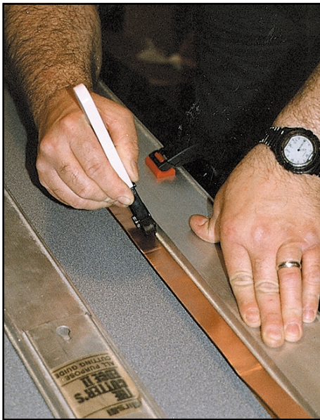
Fig 11.38 —Larry Wolfgang, WR1B, using a 4-foot straightedge designed as a guide for hand-held circular saws to clamp the copper foil tape to a board on a tabletop. After carefully measuring to ensure a uniform 22 mm width, he cut the foil tape using a Fiskars rotary cutter. Be careful to keep the cutter wheel against the straightedge for the entire length. Move the tape in 4-foot intervals to cut the entire length. (Photo by Dan Wolfgang.)
