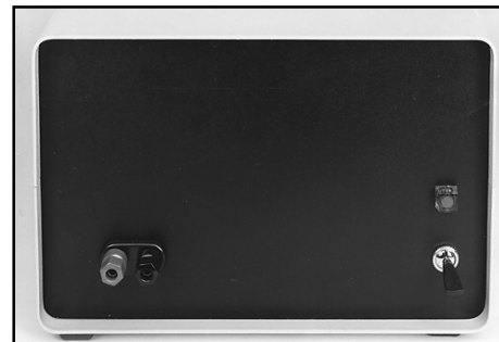
Fig 11.49 — The front panel of the 28-V power supply sports only a power switch, pilot lamp and binding posts for the voltage output. There is room for a voltmeter, should another builder desire one.
