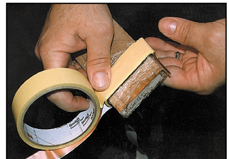
Fig 11.39 —Winding the foil tape tightly on the epoxy-coated paper bobbin on the wooden block. The mylar tape is unrolled and positioned over the foil layer as you wind. (Photo by Dan Wolfgang.)
