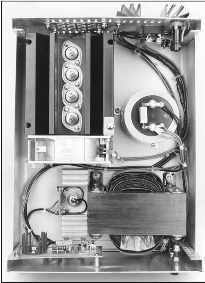
Fig 11.52 — Interior of the 28-V, high-current power supply. The cooling fan is necessary only if the pass transistors and heat sink are mounted inside the cabinet. See text.
