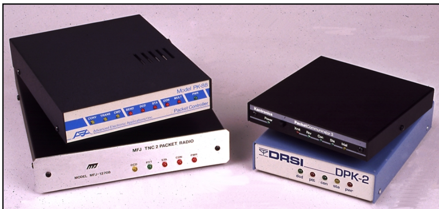
Fig 12.29 —Four popular 1200 bit/s packet TNCs: (clockwise, from left to right) the AEA PK-88, MFJ-1270C, DRSI DPK-2 and the Kantronics KPC-3.
