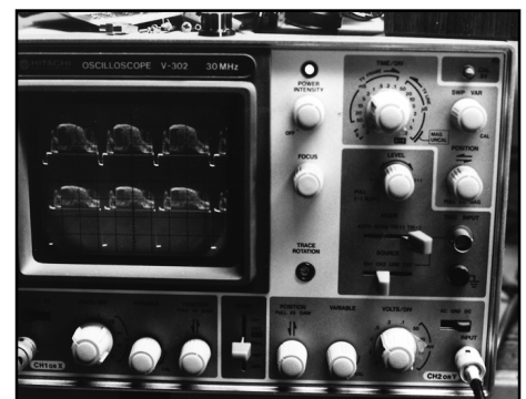
Fig 12.66—An oscilloscope used to observe a video waveform. The lower trace is the video signal as it comes out of the sync stretcher. The upper trace is the signal from the Mirage D1010-N amplifier.
