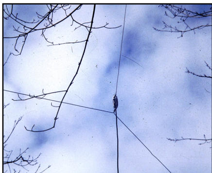
Fig 20.48 —The feedpoint of the tree-mounted groundplane antenna. The opposite ends of the two radial wires may be connected to stakes or other convenient anchor points. Make sure that the radials are high enough so that people cannot come in contact with them.
