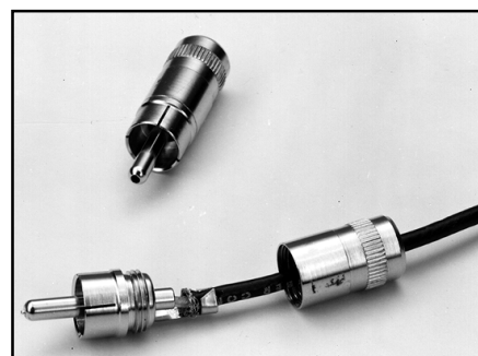
Fig 22.15 —Phono plugs have countless uses around the shack. They are small and shielded; the type with the metal body is easy to grip. Be careful not to use too much heat when soldering the ground (outer) conductor—you may melt the insulation.
