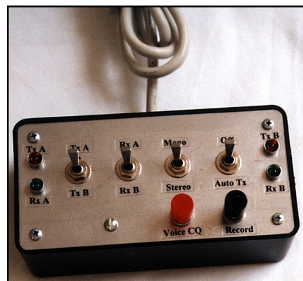
Fig 22.83 —The remote head for the Two-Radio Switchbox.
