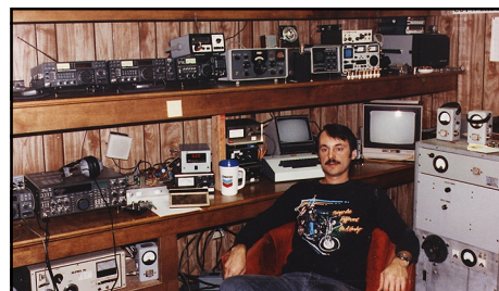
Fig 22.8 —Richard, WB5DGR, uses a homebrew 1.5-kW amplifier to seek EME contacts from this nicely laid out station.
