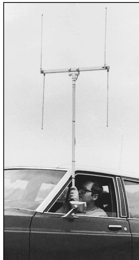
Fig 23.84 — A set of TDOA RDF antennas is light weight and mounts readily through a sedan window without excessive overhang.
