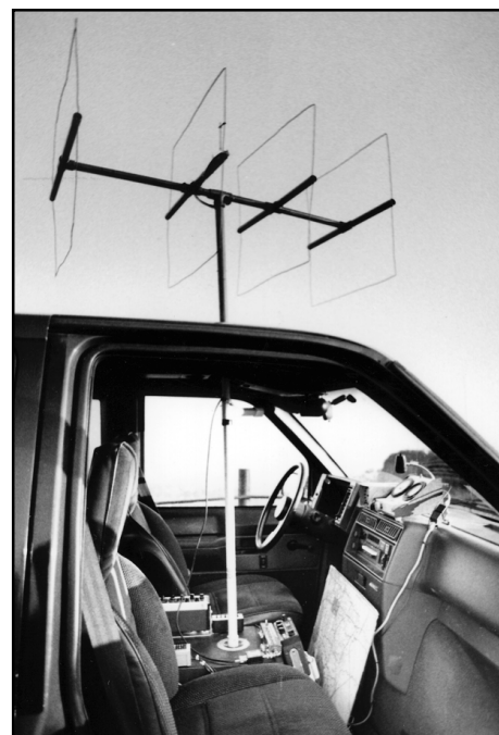
Fig 23.79 — K0OV uses this mobile setup for RDF on several bands, with separate antennas for each band that mate with a common lower mast section, pointer and 360° indicator. Antenna shown is a heavy gauge wire quad for 2 m.
