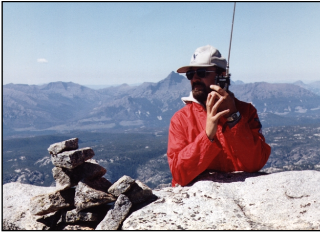
Fig 23.8 — In the Rocky Mountain west, hand-held transceivers can often cover great distances, thanks to repeaters located atop high mountains. (photo courtesy WB0KRX and N0IET)
