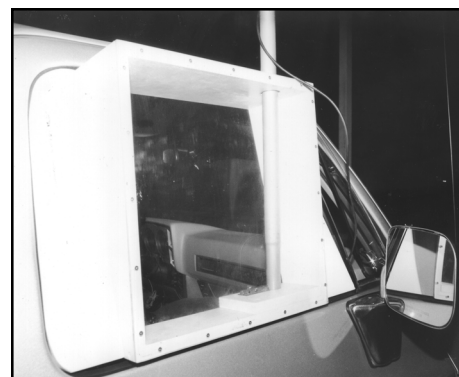
Fig 23.85 — A window box allows the navigator to turn a mast mounted antenna with ease while remaining dry and warm. No holes in the vehicle are needed with a properly designed window box.
