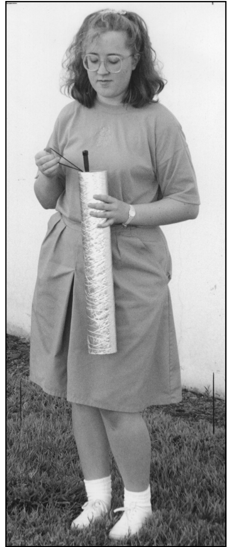
Fig 23.90 — The air attenuator for a VHF hand-held in use. Suspend the radio by the wrist strap or a string inside the tube.
