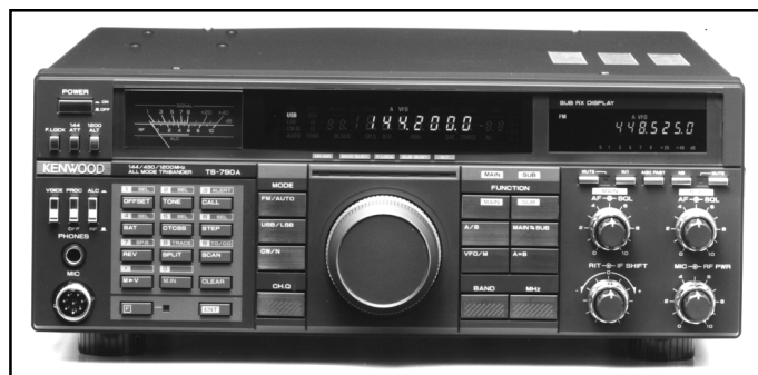
Kenwood's TS-790A is a dual-band (144-148 MHz and 430-450 MHz) multimode transceiver. A 23-cm (1240-1300 MHz) module is optional. Power output is 35-45 W on 144 MHz, 30-40 W on 430 MHz and 10 W on 1240 MHz.
