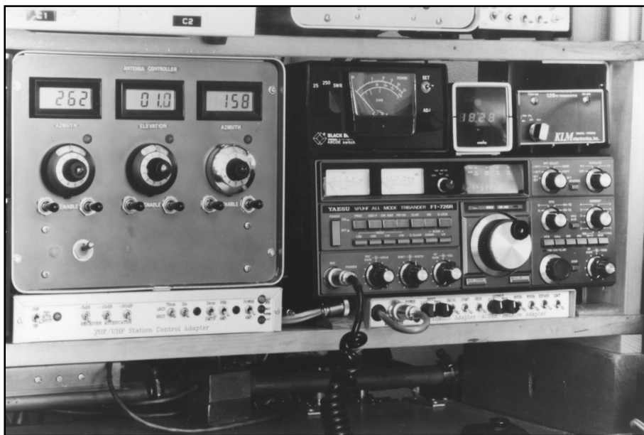
Fig 23.48 — The satellite station at WD4FAB, with a home-brew antenna controller mounted above a low-profile station controller. On the right is a Yaesu FT-726R transceiver, with a power meter, clock and 23-cm transverter mounted on top.
